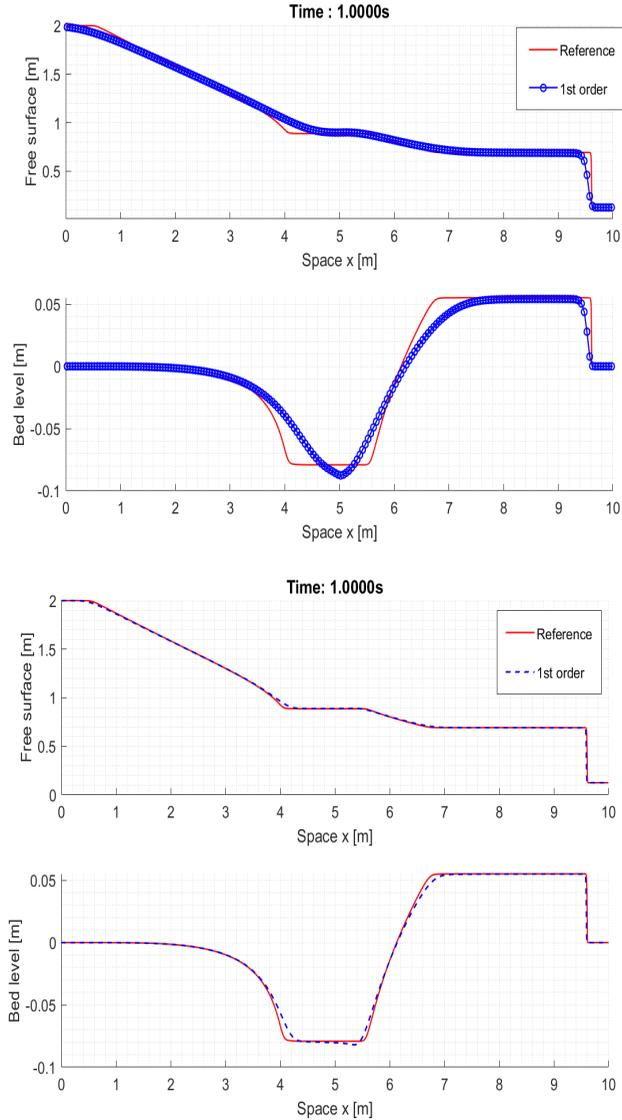
FIG. 5.1. RP: dam break on movable bottom; free surface (up) and bed level (bottom). Reference solution (red) and first-order weakly coupled solution (blue).  $M=200$  cells (up) and  $M=2000$  cells (bottom).
