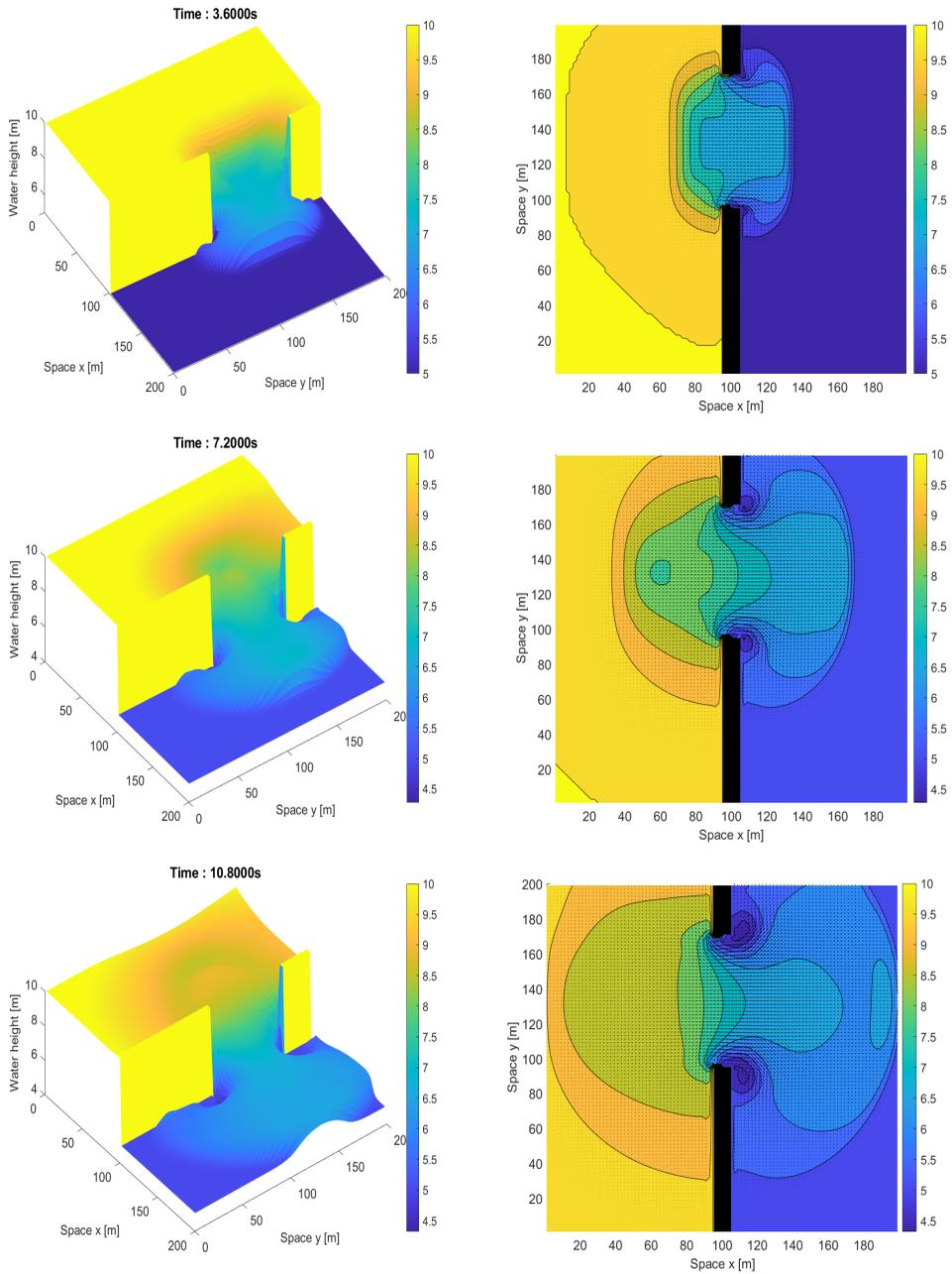
FIG. 5.9. Squared dam break; water height (left) and contour plot and velocity field (right) at time  $t = 3.6\text{ s}$  (up),  $t = 7.2\text{ s}$  (middle) and  $t = 10.8\text{ s}$  (bottom). Dam in black. 2D extension of second order scheme with  $M = 100$  cells and  $CFL = 0.25$ .
