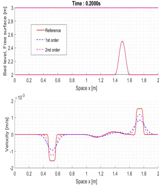
FIG. 5.5. Propagation of perturbation; bed level  $z$  and free surface  $z+h$  (top), velocity (bottom). First (blue) and second-order (magenta) weakly coupled solutions with  $M=200$  cells. Reference solution in red.
