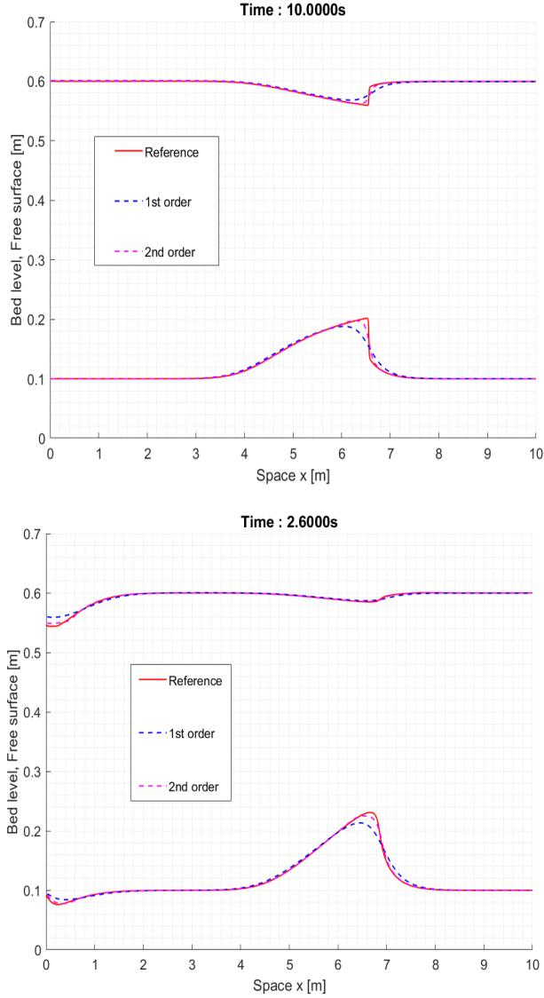
FIG. 5.3. Flow over a movable bump; bed level  $z$  and free surface  $z+h$ ;  $A_g=0.005$  (up) and  $A_g=0.07$  (bottom). First (blue) and second-order (magenta) weakly coupled solutions with  $M=200$  cells. Reference solution in red.
