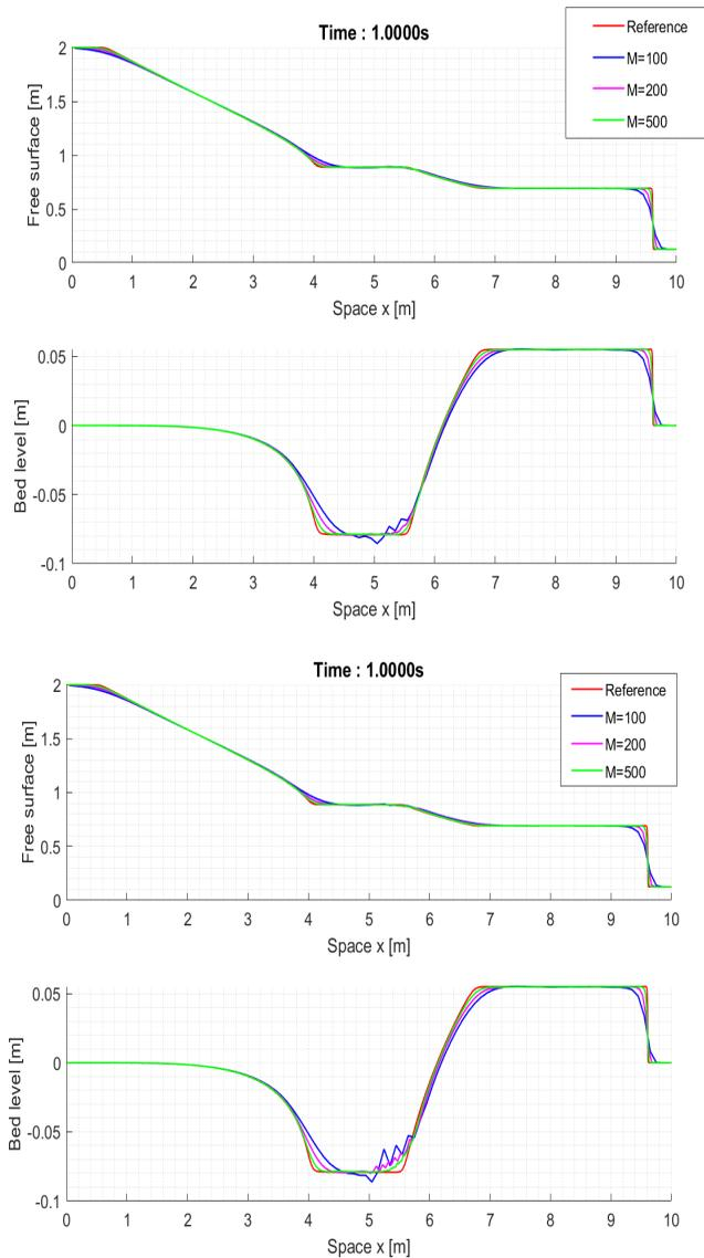
FIG. 5.2. RP: dam break on movable bottom; free surface (up) and bed level (bottom). "Decoupled" (bottom) and "weakly coupled" (up) solutions. Mesh of size  $M = 100$  (blue line),  $M = 200$  (magenta line) and  $M = 500$  (green line) cells. Red line for reference solution.
