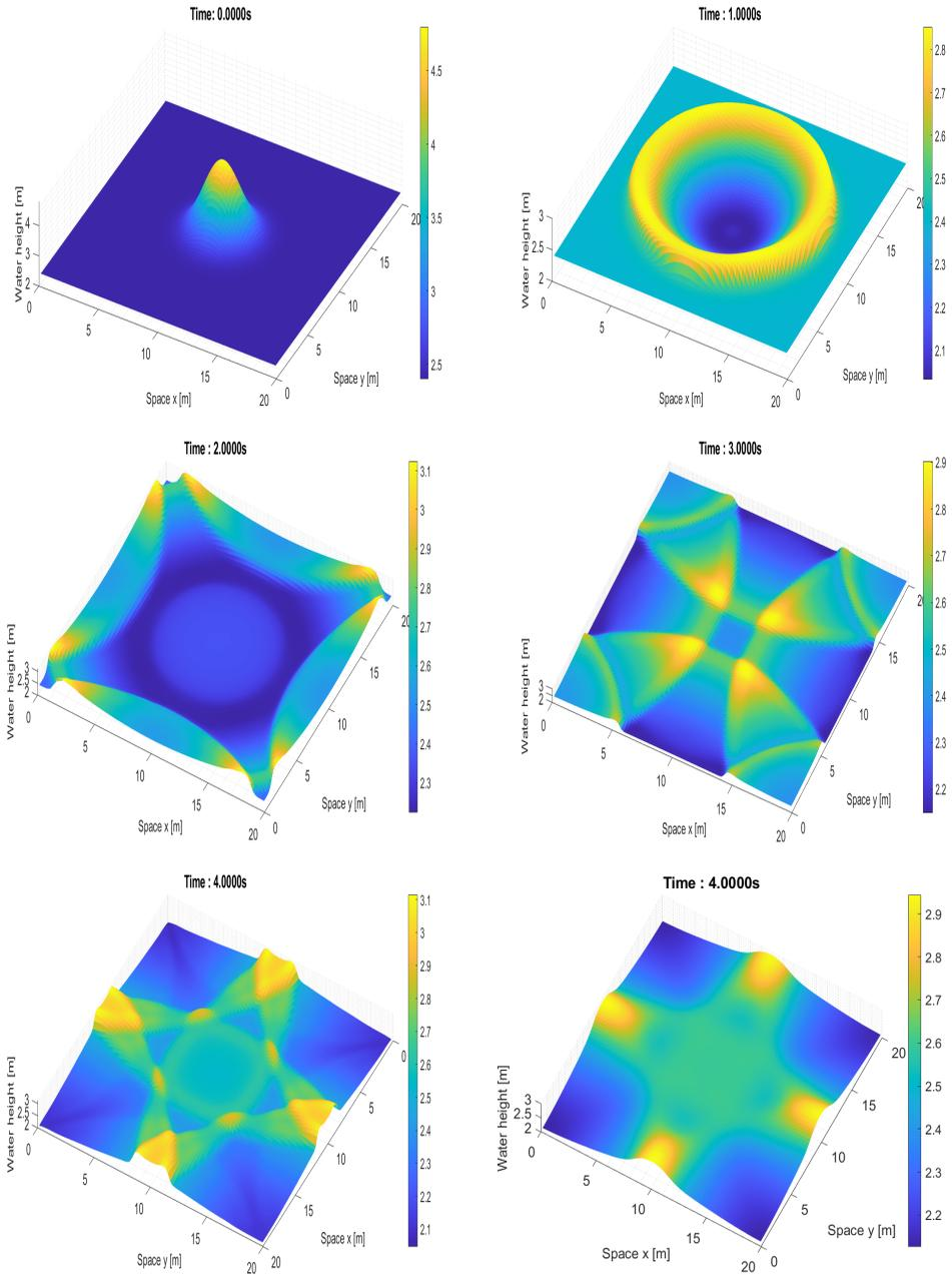
FIG. 5.7. Water drop in a basin; water height at time  $t=0s$  (up, left),  $t=1s$  (up, right),  $t=2s$  (middle, left),  $t=3s$  (middle, right) and  $t=4s$  (bottom).  $M=100$  cells,  $CFL=0.25$  and  $CFL=0.45$  for the 2D extension of second and first order scheme respectively. 2D-extension of the 1D first-order scheme used only in the image on the bottom-right.
