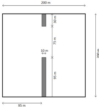
FIG. 5.8. Geometry of the dam in the squared dam break test problem.
