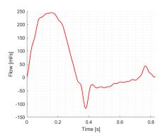
Figure 40: Heart flow imposed at the beginning of the ascending aorta.
