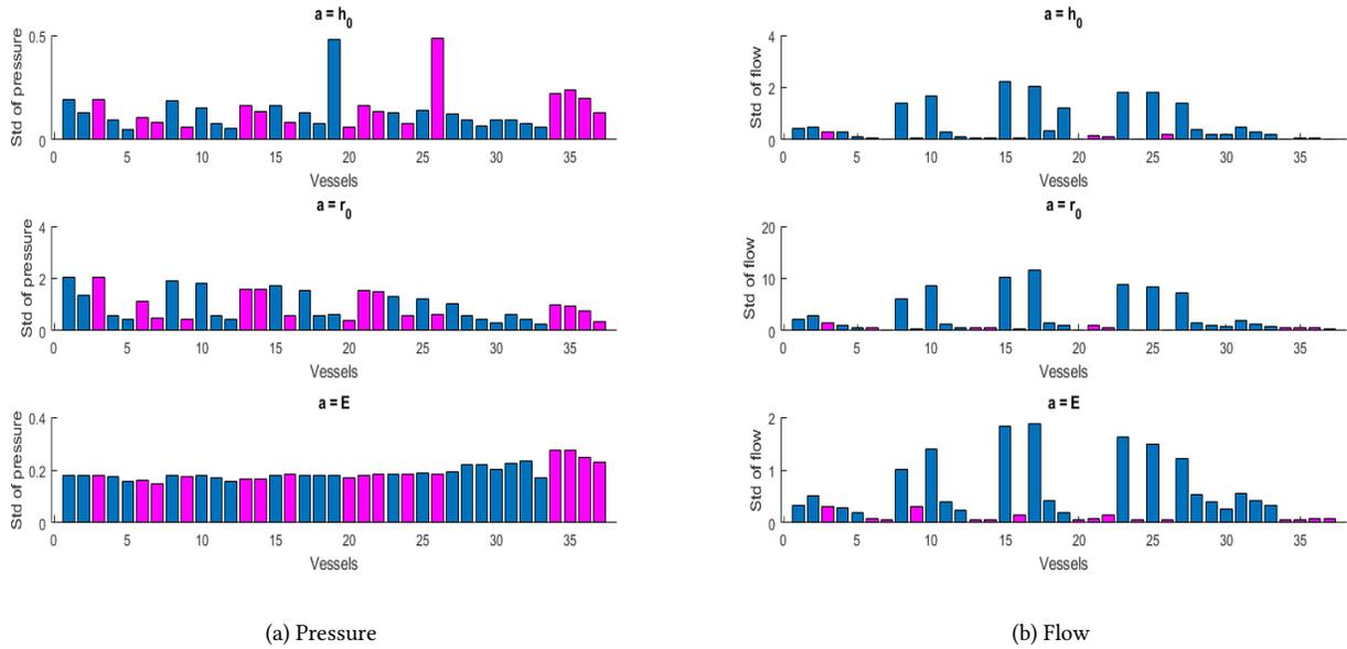
Figure 48: Maximum absolute value of standard deviation of pressure (left) and flow (right) using  $a = h_0$  (top),  $a = r_0$  (middle) and  $a = E$  (bottom) in the midpoint of each vessels of the network (identified with numbers from 1 to 37). Magenta color for terminal vessels. Viscoelastic case, MUSCL-Hancock method.
