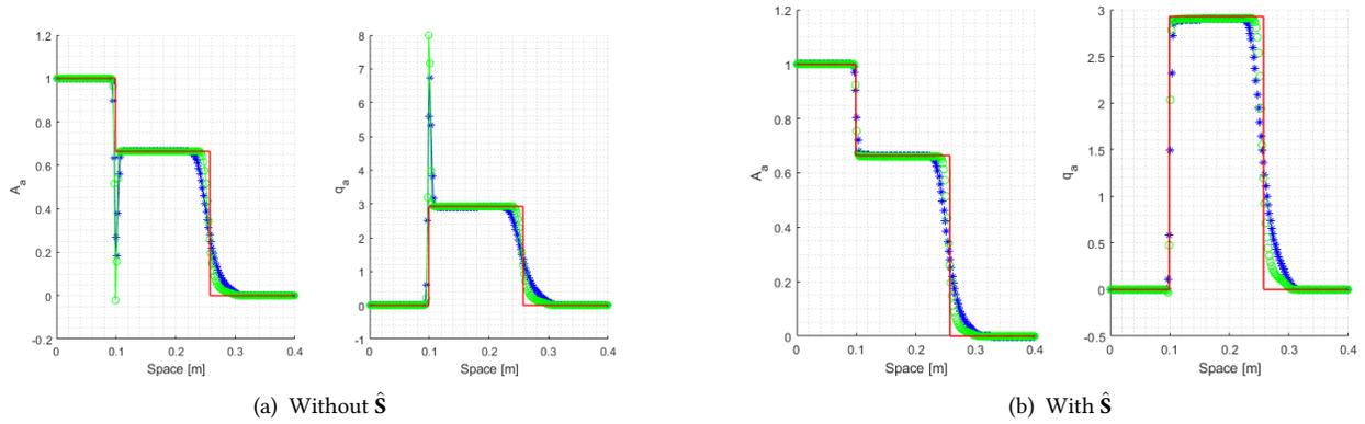
Figure 8: Comparison among Price-T (blue symbol ‘\*’), MUSCL-Hancock (green symbol ‘o’) and exact solution (red line). Derivative of the area  $A_a$  and flux  $q_a$  with  $a = A_L$  for test 1 of table 2. Mesh with  $M = 200$  cells,  $\Gamma = 0$ .
