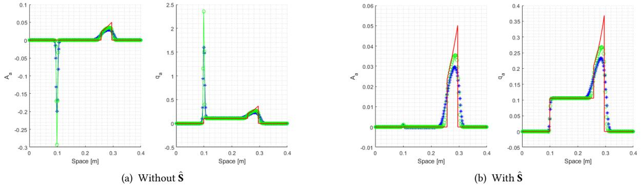
Figure 11: Comparison among Price-T (blue symbol '\*'), MUSCL-Hancock (green symbol 'o') and exact solution (red line). Derivative of the area  $A_\alpha$  and flux  $q_\alpha$  with  $a = r_0$  for test 1 of table 2. Mesh with  $M = 200$  cells,  $\Gamma = 0$ .
