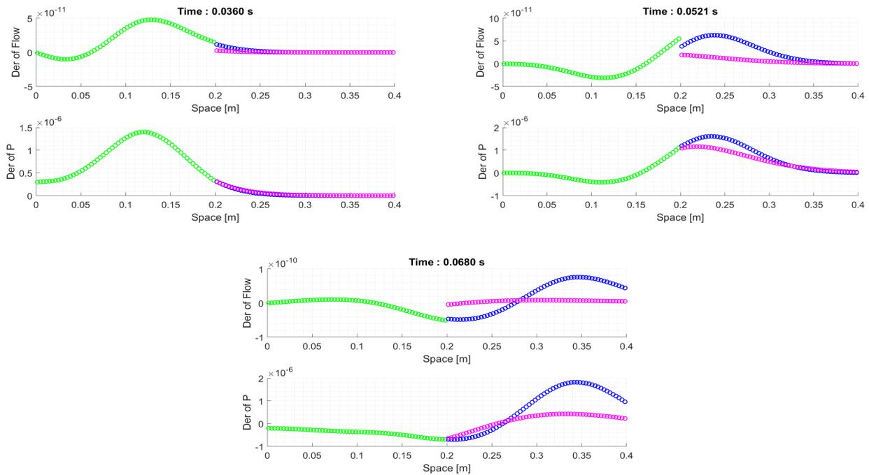
Figure 39: Derivative of flow and pressure with respect to  $a = E$  obtained with MUSCL-Hancock method. Green, blue and magenta symbols represent  $v_2$ ,  $v_3$  and  $v_4$  respectively. Mesh with  $M = 60$  cells for each vessel.
