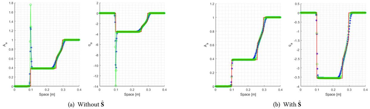
Figure 9: Comparison among Price-T (blue symbol ‘\*’), MUSCL-Hancock (green symbol ‘o’) and exact solution (red line). Derivative of the area  $A_a$  and flux  $q_a$  with  $a = A_R$  for test 1 of table 2. Mesh with  $M = 200$  cells,  $\Gamma = 0$ .
