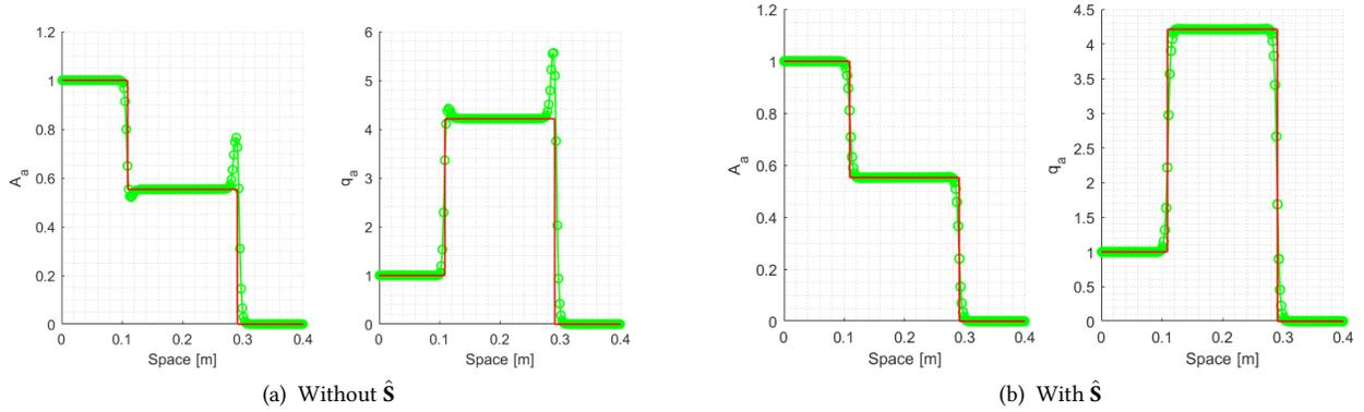
Figure 15: Comparison between MUSCL-Hancock (green symbol 'o') and exact solution (red line). Derivative of the area  $A_a$  and flux  $q_a$  with  $a = A_L$  for test 3 of table 2. Mesh with  $M = 200$  cells,  $\Gamma = 0$ , CFL = 0.5.
