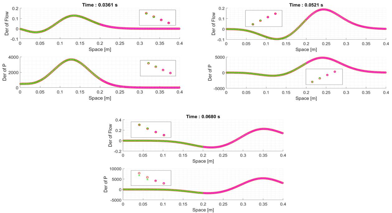
Figure 33: Derivative of flow and pressure with respect to  $a = h_0$  obtained MUSCL-Hancock method. Red symbol 'o' for the unique vessel, green and magenta symbol 'x' for the two coupled vessels. Mesh with  $M = 120$  cells for the unique vessel.
