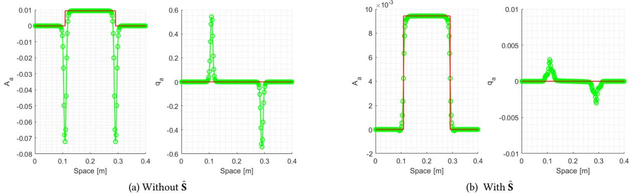
Figure 18: Comparison between MUSCL-Hancock (green symbol 'o') and exact solution (red line). Derivative of the area  $A_a$  and flux  $q_a$  with  $a = r_0$  for test 3 of table 2. Mesh with  $M = 200$  cells,  $\Gamma = 0$ , CFL = 0.5.
