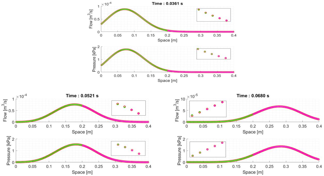
Figure 32: Flow and pressure obtained with MUSCL-Hancock method. Red symbol 'o' for the unique vessel, green and magenta symbol 'x' for the two coupled vessels. Mesh with  $M = 120$  cells for the unique vessel.
