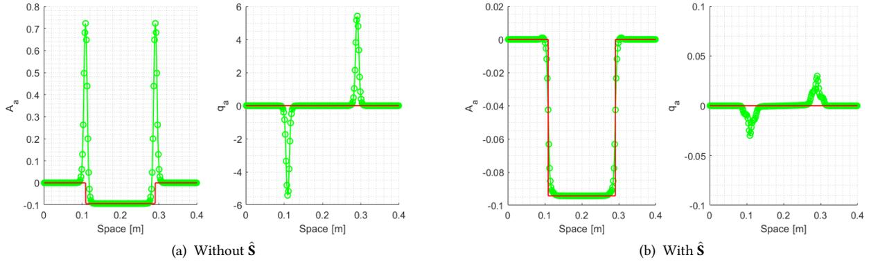
Figure 17: Comparison between MUSCL-Hancock (green symbol 'o') and exact solution (red line). Derivative of the area  $A_a$  and flux  $q_a$  with  $a = h_0$  for test 3 of table 2. Mesh with  $M = 200$  cells,  $\Gamma = 0$ , CFL = 0.5.
