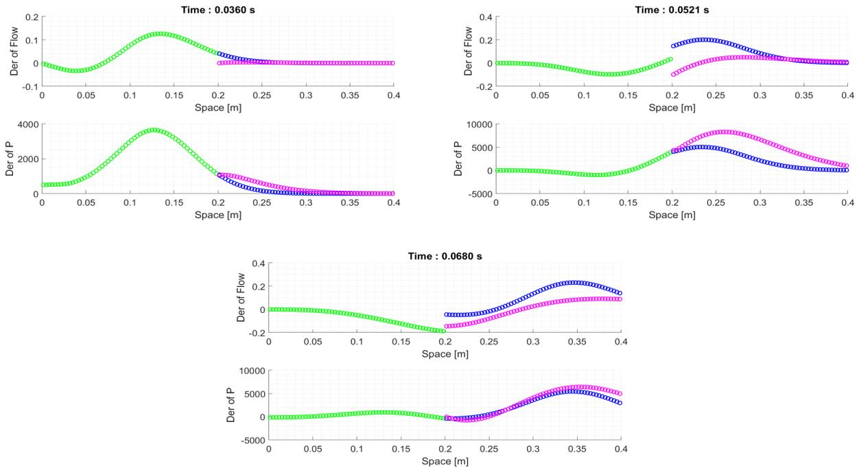
Figure 37: Derivative of flow and pressure with respect to  $a = h_0$  obtained MUSCL-Hancock method. Green, blue and magenta symbols represent  $v_2$ ,  $v_3$  and  $v_4$  respectively. Mesh with  $M = 60$  cells for each vessel.
