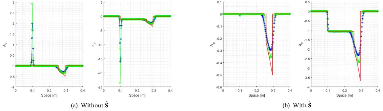
Figure 10: Comparison among Price-T (blue symbol '\*'), MUSCL-Hancock (green symbol 'o') and exact solution (red line). Derivative of the area  $A_\alpha$  and flux  $q_\alpha$  with  $a = h_0$  for test 1 of table 2. Mesh with  $M = 200$  cells,  $\Gamma = 0$ .
