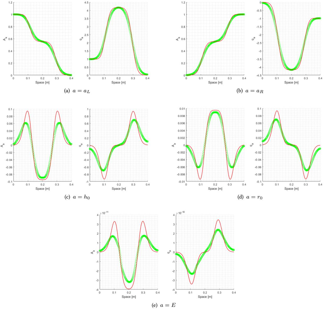
Figure 22: MUSCL-Hancock solution computed using a mesh with  $M = 200$  cells (green symbol 'o') and with  $M = 2000$  cells (red line). Derivative of the area  $A_a$  and flux  $q_a$  for test 3 of table 2.  $\Gamma = 1 \text{ Pa s m}$ .
