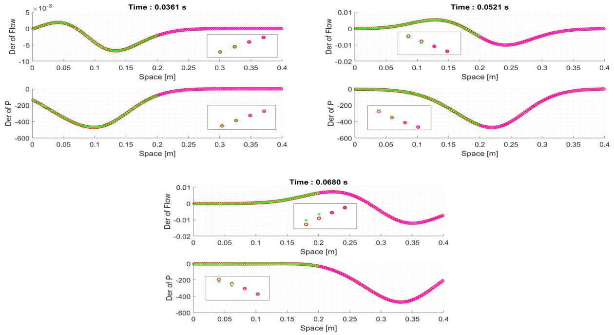
Figure 34: Derivative of flow and pressure with respect to  $a = r_0$  obtained with MUSCL-Hancock method. Red symbol 'o' for the unique vessel, green and magenta symbol 'x' for two coupled vessels. Mesh with  $M = 120$  cells for the unique vessel.
