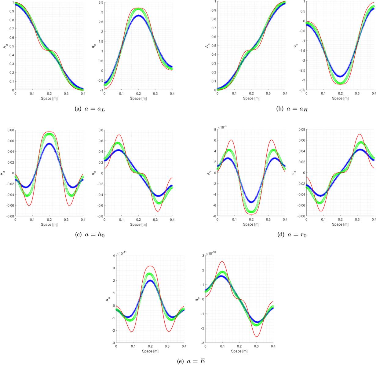
Figure 21: MUSCL-Hancock solution computed using a mesh with  $M = 200$  cells (green symbol 'o') and with  $M = 2000$  cells (red line). Derivative of the area  $A_a$  and flux  $q_a$  for test 2 of table 2.  $\Gamma = 1 \text{ Pa s m}$ .
