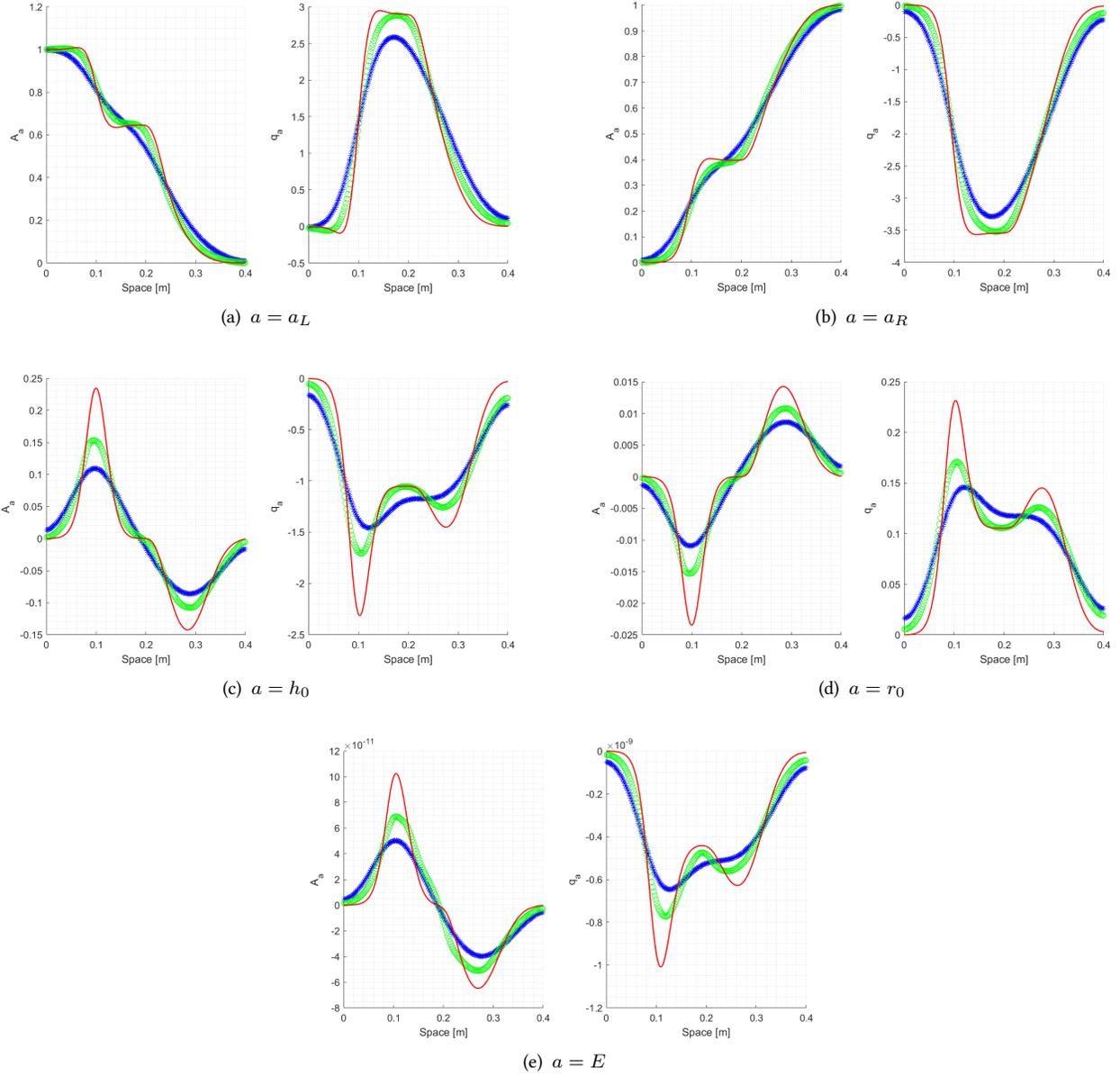
Figure 20: Price-T (blue symbol '\*') and MUSCL-Hancock (green symbol 'o') solution computed using a mesh with  $M = 200$  cells, reference solution (red line) with  $M = 2000$  cells. Derivative of the area  $A_a$  and flux  $q_a$  for test 1 of table 2.  $\Gamma = 1 \text{ Pa s m}$ .
