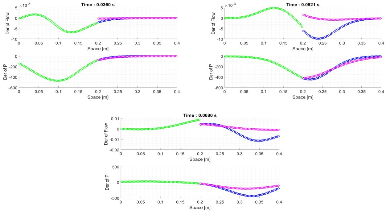
Figure 38: Derivative of flow and pressure with respect to  $a = r_0$  obtained with MUSCL-Hancock method. Green, blue and magenta symbols represent  $v_2$ ,  $v_3$  and  $v_4$  respectively. Mesh with  $M = 60$  cells for each vessel.
