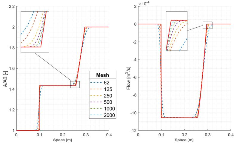
(a) Test 1 - Left shock, right rarefaction
