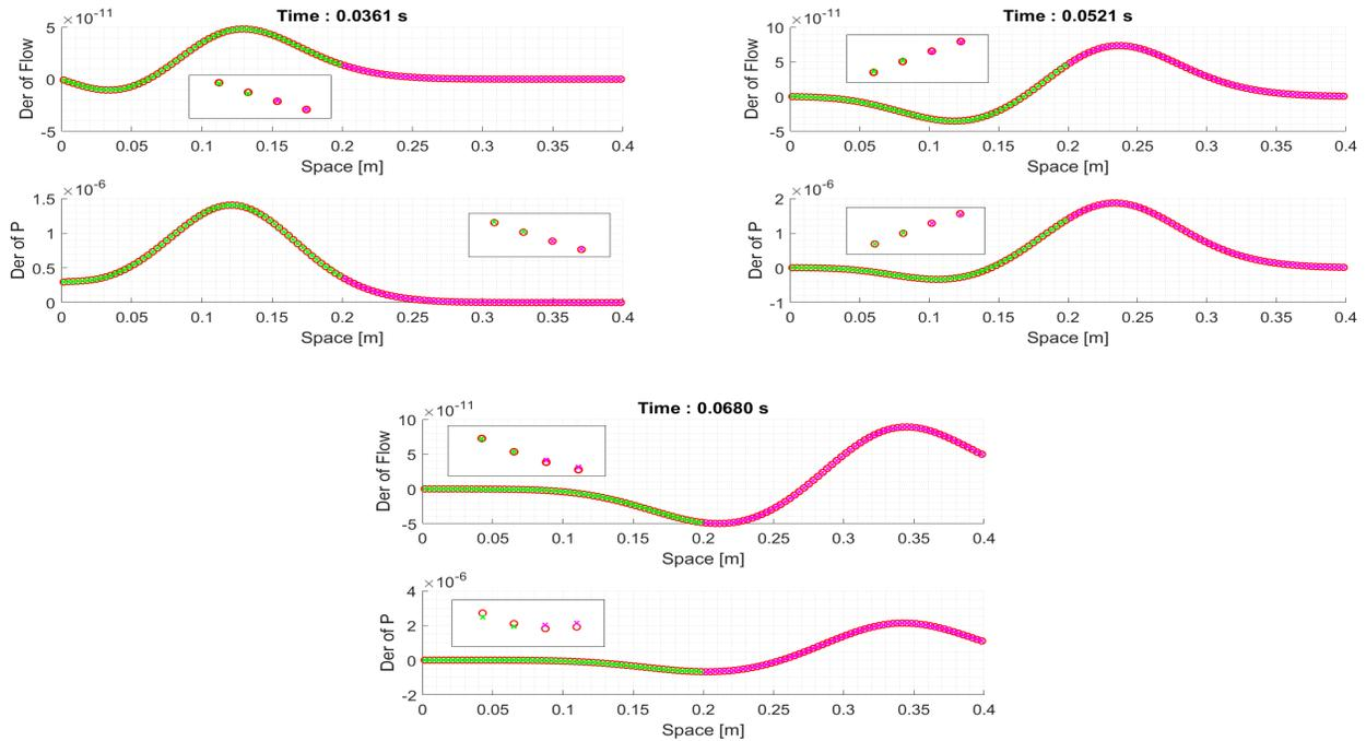
Figure 35: Derivative of flow and pressure with respect to  $a = E$  obtained with MUSCL-Hancock method. Red symbol 'o' for the unique vessel, green and magenta symbol 'x' for two coupled vessels. Mesh with  $M = 120$  cells for the unique vessel.
