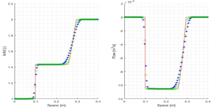
(a) Test 1 - Left shock, right rarefaction
