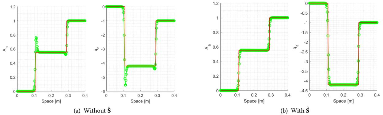
Figure 16: Comparison between MUSCL-Hancock (green symbol 'o') and exact solution (red line). Derivative of the area  $A_a$  and flux  $q_a$  with  $a = A_R$  for test 3 of table 2. Mesh with  $M = 200$  cells,  $\Gamma = 0$ , CFL = 0.5.
