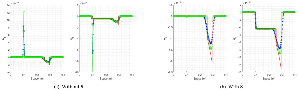
Figure 12: Comparison among Price-T (blue symbol '\*'), MUSCL-Hancock (green symbol 'o') and exact solution (red line). Derivative of the area  $A_\alpha$  and flux  $q_\alpha$  with  $a = E$  for test 1 of table 2. Mesh with  $M = 200$  cells,  $\Gamma = 0$ .
