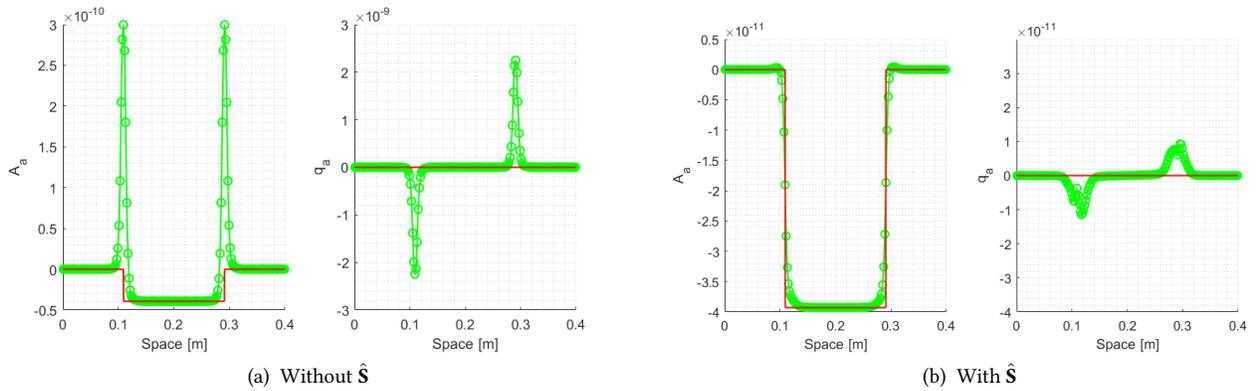
Figure 19: Comparison between MUSCL-Hancock (green symbol 'o') and exact solution (red line). Derivative of the area  $A_a$  and flux  $q_a$  with  $a = E$  for test 3 of table 2. Mesh with  $M = 200$  cells,  $\Gamma = 0$ , CFL = 0.5.
