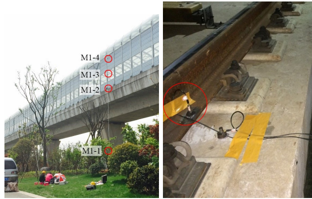
(a) The microphones (b) The piezoelectric acceleration sensor
