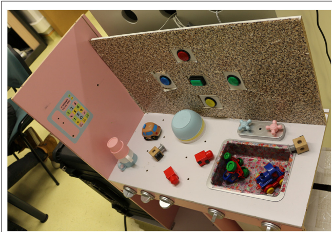
FIGURE 7 | The setup used for all the experiments. The setup is a toy kitchen with 5 interactive push buttons integrated into a vertical plane.
