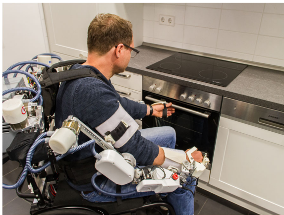
Fig. 3 An upper-body exoskeleton integrated into a wheel chair can support patients in doing everyday tasks as well as the overall rehabilitation process. (Copyright: DFKI GmbH)
