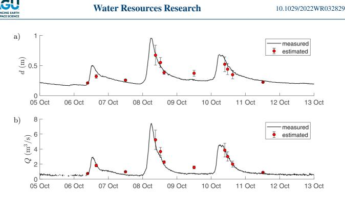
Figure 15. Temporal evolution of the measured (black line) and estimated (red circles) water (a) depth and (b) discharge of the River Calder, between 5 October and 13 October 2020. The error bars represent the uncertainty estimated with synthetic data.
