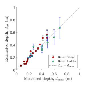
**Figure 12.** Water depth estimated from videos of the River Sheaf (red) and Calder (blue). The abscissa is the measured water depth,  $d_{\text{meas}}$ . The dashed line indicates  $d_{\text{est}} = d_{\text{meas}}$ . The error bars represent the uncertainty estimated with synthetic data.
