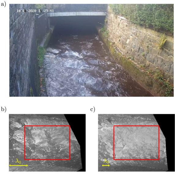
**Figure 9.** (a) A snapshot of a video of the River Calder (flow condition C08). (b and c) Examples of orthorectified images recorded in flow condition (b) C08 and (c) C02. The red square indicates the borders of the area used for the analysis.  $\lambda_0$  is the characteristic wavelength estimated by Equation 8.
