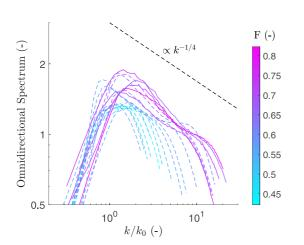
**Figure 11.** Omnidirectional spatial spectra of the image intensity. (dashed), River Sheaf and (solid), River Calder.  $k_0$  is the characteristic wavenumber according to Equation 8. Only the flow conditions with  $\lambda_0 < L_{min}/2$  are shown.
