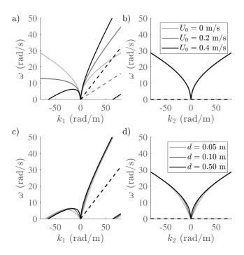
**Figure 2.** Effect of (a and b) flow velocity and (c and d) depth on the frequency of (solid lines) gravity-capillary waves and (dashed lines) turbulence-generated surface deformations. (a and c) Waves are parallel to the flow direction,  $k = k_1$ ,  $k_2 = 0$ . (b and d) Waves are perpendicular to the flow direction,  $k = k_2$ ,  $k_1 = 0$ . Example calculated for m = 0.34. (a and b) d = 0.5 m. (c and d),  $U_0 = 0.4$  m/s.
