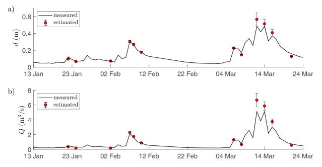
Figure 14. Temporal evolution of the measured (black line) and estimated (red circles) water (a) depth and (b) discharge of the River Sheaf, between 13 January and 23 March 2019. The measured discharge has been calculated by means of the fitted rating curve, as a function of the measured depth. The error bars represent the uncertainty estimated with synthetic data.
