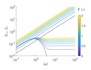
**Figure 6.** Nondimensional sensitivity parameters, which indicate the sensitivity of the waves dispersion relation with respect to (solid) speed variations,  $\xi_{U_0}$ , and (dashed) depth variations,  $\xi_d$ . Data are expressed as a function of the nondimensional wavenumber kd and Froude number F. An example calculated with m = 0.34, in the B  $\rightarrow \infty$  gravity waves limit.
