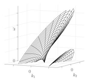
**Figure 1.** 3D Dispersion relation of gravity-capillary waves, Equation 6. Here,  $k_1$  is in the direction of the flow.
