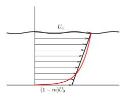
**Figure 4.** Schematic of the linear vertical profile of the streamwise velocity (black), compared to a power-function profile (red). The linear profile has m = 0.34. The power-function profile has  $\eta = 0.2048$ . Both profiles have a velocity index  $\alpha = 0.83$ .
