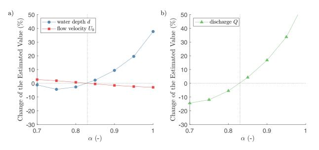
**Figure 5.** Relative variation of the estimated flow parameters as a function of the assumed velocity index  $\alpha$ . The relative changes are with respect to the estimations obtained with  $\alpha = 0.83$ . Variations of the estimated depth and surface velocity (a) are due to the dependence of the velocity gradient *m* on  $\alpha$  through Equation 16. Variations of the discharge (b) are due also to the direct dependence on  $\alpha$  according to Equation 2.
