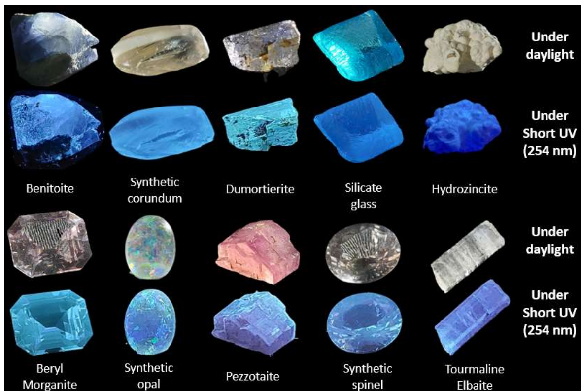
Figure 1. Photo under daylight and under shortwave UV (254 nm) of the ten representative samples of BSL phenomena. (Photo: Maxence Vigier).
