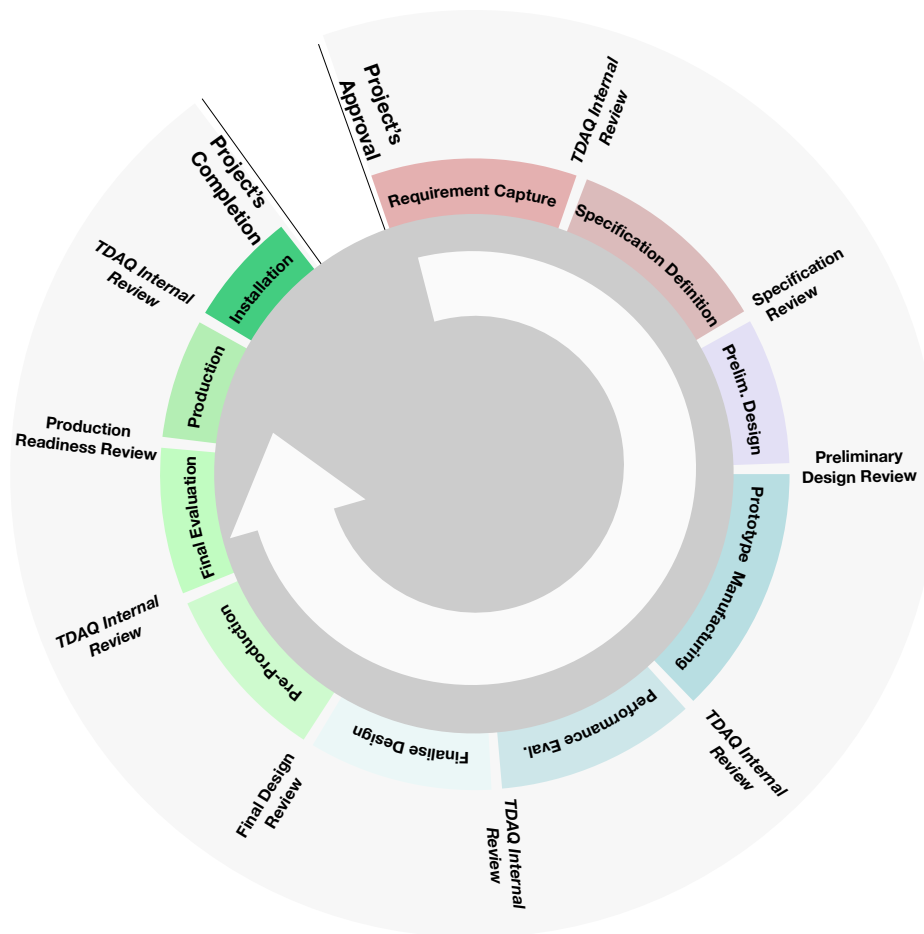
Figure 19.1: Sequence of activities and approval reviewing processes at different stages of the development and of the production cycle of any project's deliverable.
