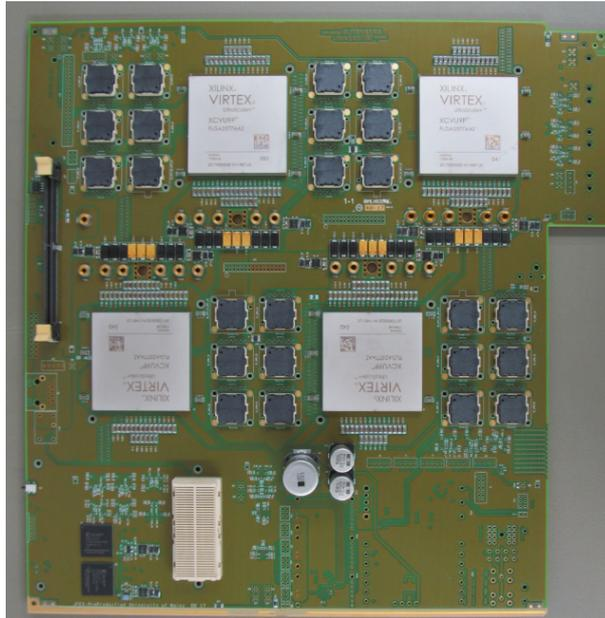
Figure 7.8: Photograph of the final prototype of a *jFEX* blade. The board is equipped with four high speed grade FPGAs and the minipod connectors for the optical input and output. Missing on this module are various infrastructure components for control and power management of the board.
