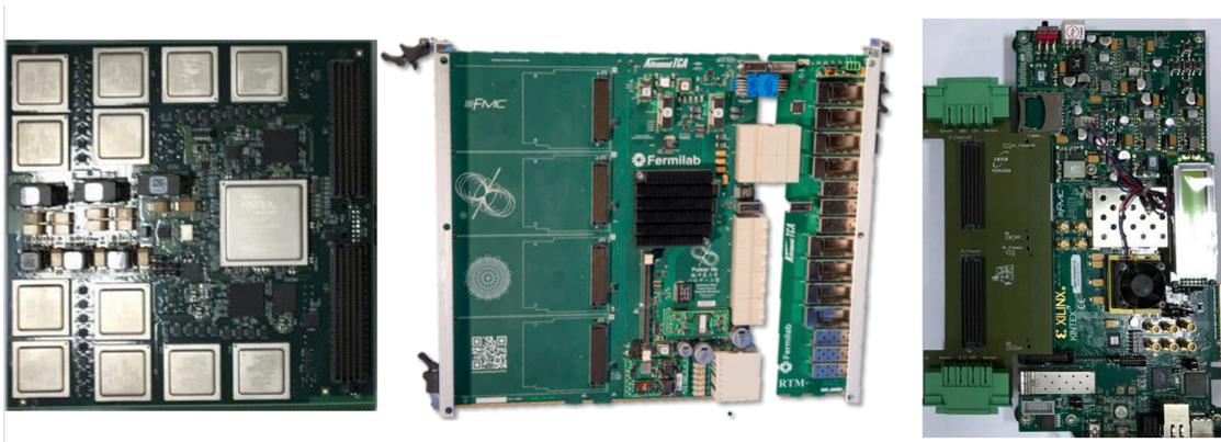
Figure 13.14: Hardware demonstration prototypes based on current-generation devices: *AM mezzanine with Kintex Ultrascale FPGA (left), ATLAS Data Organiser ATCA carrier for FMC mezzanine cards based on a Virtex 7 FPGA (middle), and a Virtex 7 FPGA evaluation board equipped with a mechanical adapter to host the AM mezzanine card.*
