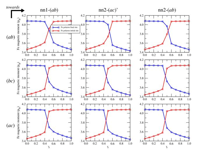
FIG. 6: Spin magnetic moment on the two Fe involved in the nine polaronic hopping of Fig. 5. The initial and final values ( $\approx 4.08$  and 3.43-3.46  $\mu_B$ ) respectively correspond to Fe<sup>3+</sup> and Fe<sup>4+</sup>.
