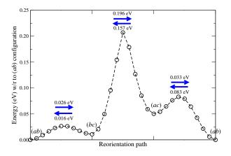
FIG. 4: Energy profile for the three onsite-reorientations of the self-trapped hole polaron, from (ab) to (bc), from (bc) to (ac) and from (ac) to (ab), with the corresponding energy barriers. The energy of (ab) is taken as reference.
