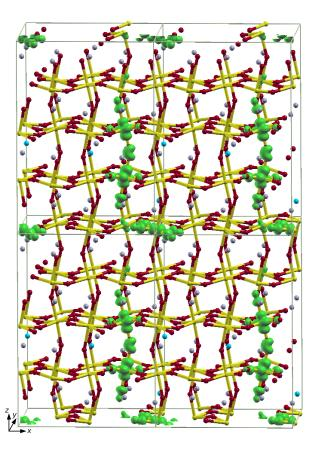
FIG. 8: Configuration of  $\text{La}_{1-x}\text{Sr}_x\text{FeO}_3$  with  $x \approx 0.1$ , with isosurfaces ( the isovalue is 0.05  $e/\text{Å}^3$ ) of the three hole states, as obtained from the HSE06 structural optimization. The three holes are localized and close to the Sr impurities (blue circles). The supercell is doubled twice along x and z for a better view of the hole states.
