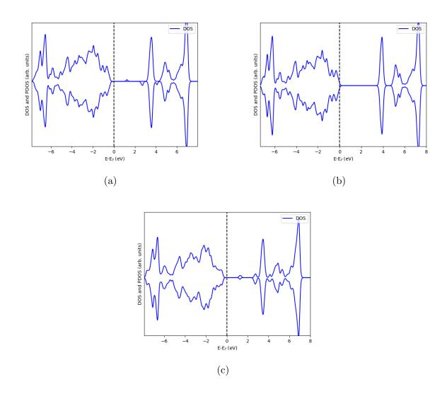
FIG. 2: Electronic densities of states of (a) the LF supercell with a self-trapped hole polaron, (b) the same supercell with a delocalized hole, and (c) the LSF supercell with  $x \approx$ 0.1, as obtained using the HSE06 functional. The Fermi energy is set at 0 eV.
