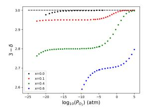
FIG. 14: Oxygen content 3- $\delta$  as a function of partial oxygen pressure  $P_{O_2}$  for x = 0,  $x \approx 0.1, 0.4$  and 0.6 at 1073 K
