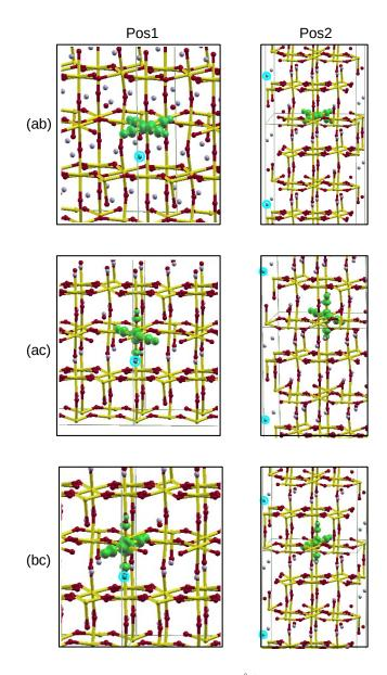
FIG. 9: The isosurfaces (the isovalue is 0.05 e/Å<sup>3</sup>) of six configurations with one Sr impurity and its associated hole, localized on two sites (Pos1: close to Sr; Pos2: far from Sr) and along the three possible orientations: (ab), (ac) and (bc). The Sr atom is in blue, and surrounded with a light blue circle for better visibility.
