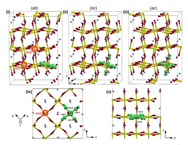
FIG. 3: (i),(ii) and (iii): Isosurfaces of electron charge density (the isovalue is  $0.05 \text{ e/Å}^3$ ) of the three possible configurations of the self-trapped hole polaron in the orthorhombic crystal LaFeO<sub>3</sub>. z is the apical direction. (iv), (v): two other views of configuration (ab) where the hole polaron lies along the equatorial plane. Fe-O distances within the polaron are indicated on panel (iv).
