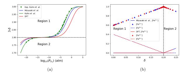
FIG. 13: (a) Oxygen concentration (3- $\delta$ ) as a function of oxygen partial pressure  $P_{O_2}$  and (b) concentrations of irons in different oxidation states as a function of oxygen nonstoichiometry at 1073 K for  $x \approx 0.4$ .
