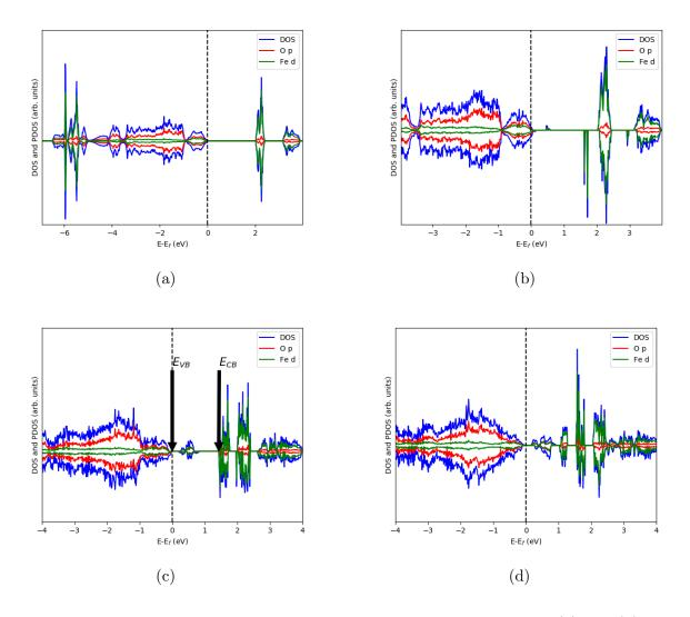
FIG. 1: Total and projected density of states obtained by GGA+U for (a) LF, (b) LSF with  $x \approx 0.1$ , (c)  $x \approx 0.4$  and (d)  $x \approx 0.6$  imposing a G-type AFM arrangement of the Fe magnetic moments. The energy scale is relative to the Fermi energy (E<sub>f</sub>=0) and the DOS
