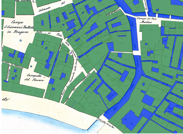
Figure 6: Example of false extraction of streets and canals (in blue)
