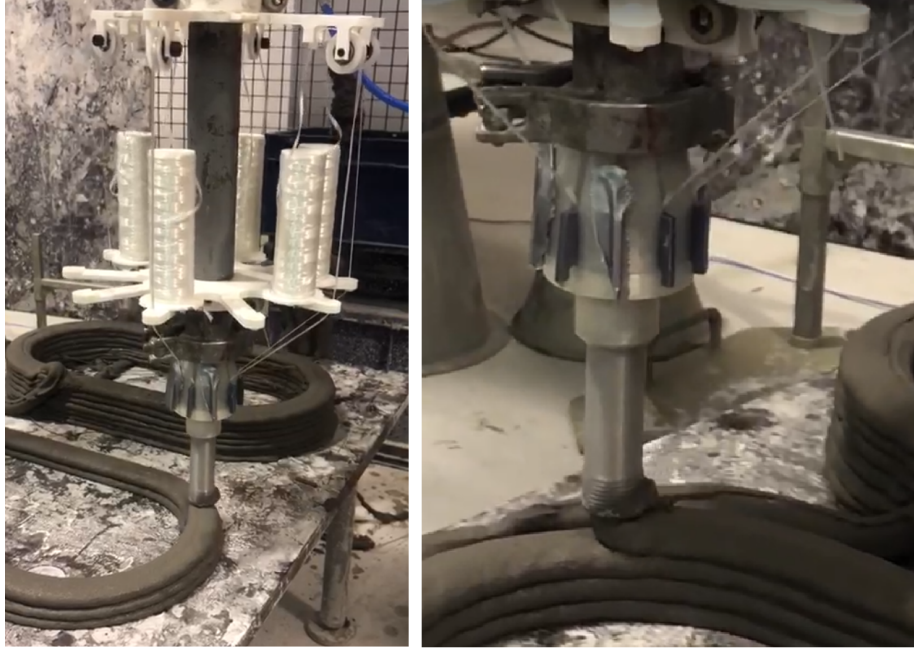
Figure 10: 3d printing of anisotropic concrete.
