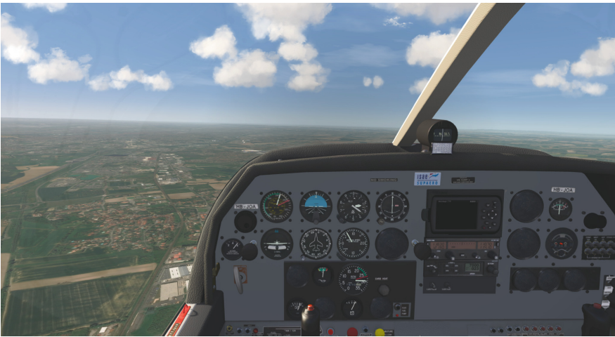
Fig. 3. DR400 cockpit panel identically reproduced in virtual reality.
