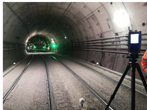
Figure 1: TLS data acquisition in low lighting conditions
