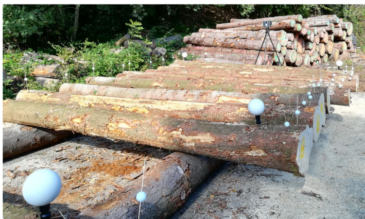
Fig. 6 A set of logs ready for T-LiDAR scanning and T-LiDAR device in place at location 3
