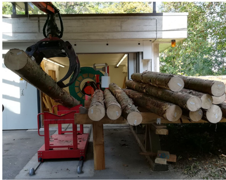
Fig. 8 Installation of a log for CT scanning
