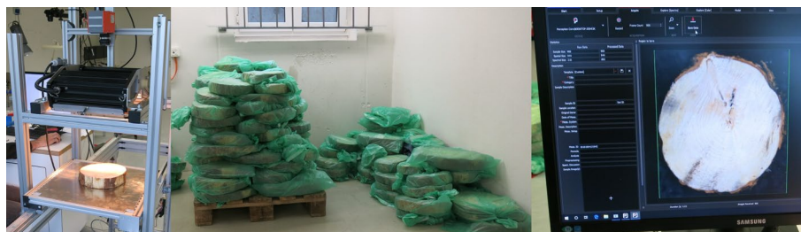
(a) Scanning system (b) Wood disc storage (c) Hyperspectral cube cropping
