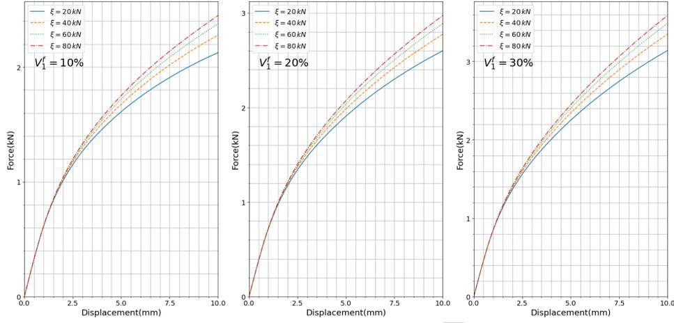
Figure 20: Force-displacement curves for the asymmetrically notched composite structure under  $5 \text{ mm s}^{-1}$  monotonic loading rate in different  $\xi^{nl}$  with  $\gamma^{nl} = 5 \text{ GPa}$  when  $V_1^f = 10\%$ ,  $V_1^f = 20\%$ ,  $V_1^f = 30\%$ . The element type is the coupled temperature-displacement brick element (C3D8T).
