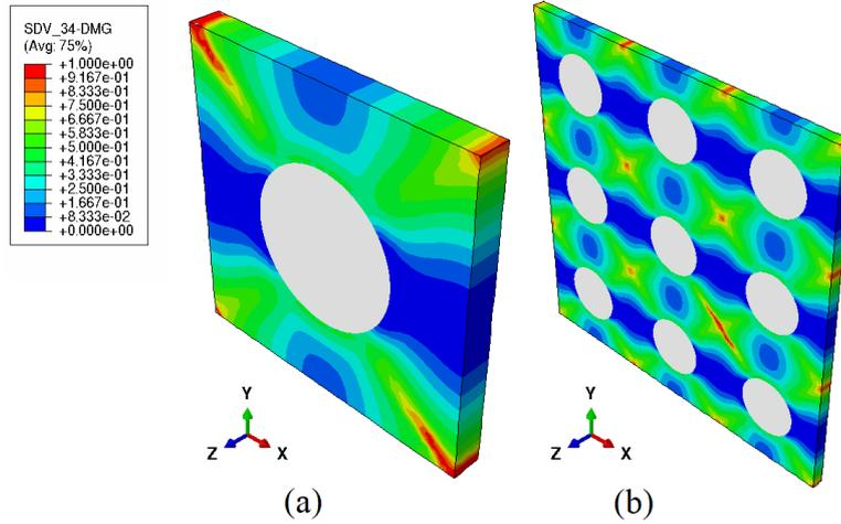
Figure 2: Damage profile under  $0.1 \text{ mms}^{-1}$  monotonic loading rate when  $l^{nl} = 0.01 l^\varepsilon$  in a) single long fiber reinforced RVE, b) a group of RVEs. Element size is set to  $0.05 \text{ mm}$ .
