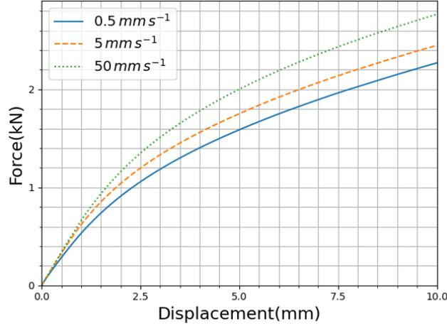
Figure 17: Force-displacement curves under different monotonic loading rates for the asymmetrically notched composite structure with  $\gamma^{nl} = 5$  GPa and  $\xi^{nl} = 80$  kN when  $V_1^f = 10\%$ . The element type is the coupled temperature-displacement brick element (C3D8T).
