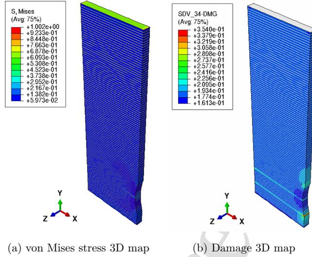
Figure 9: 3D maps of von Mises stress and damage under  $5 \text{ mms}^{-1}$  monotonic loading rate in the multi-layered structure when  $l^{nl}/l^\varepsilon \approx 36.51$ . The element type is the coupled temperature-displacement brick element (C3D8T).
