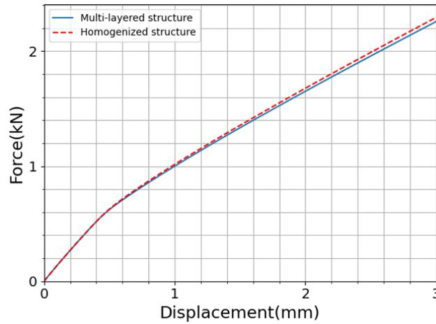
Figure 10: Force-displacement curve under  $1.5 \text{ mm s}^{-1}$  monotonic loading rate for multi-layered and homogenized unilateral notched structure using the nonlocal framework when  $l^{nl}/l^\varepsilon \approx 36.51$ ,  $\xi^{nl} = 600 \text{ kN}$ , and  $\gamma^{nl} = 5 \text{ GPa}$ .
