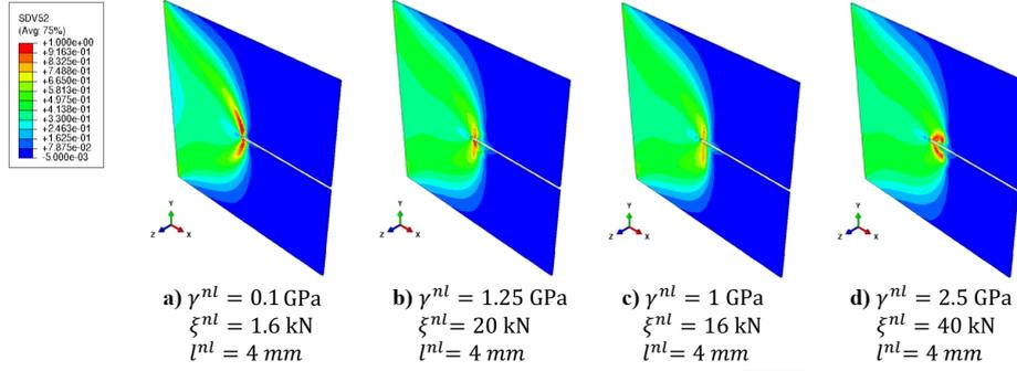
Figure 13: Matrix damage profile under  $5 \text{ mm s}^{-1}$  monotonic tensile loading using the nonlocal model with different  $\xi^{nl}$  and  $\gamma^{nl}$  when the length scale is constant ( $l^{nl} = 4 \text{ mm}$ ). The element type is the coupled temperature-displacement brick element (C3D8T).
