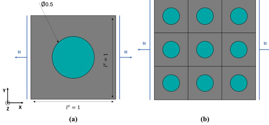
Figure 1: Loading conditions ( $\dot{\mathbf{u}} = 0.1 \text{ mms}^{-1}$ ) and the dimensions corresponding to: a) single long fiber reinforced RVE, b) a group of RVEs (dimensions are based on  $\text{mm}$ ); the thickness for both cases is  $0.1 \text{ mm}$ .
