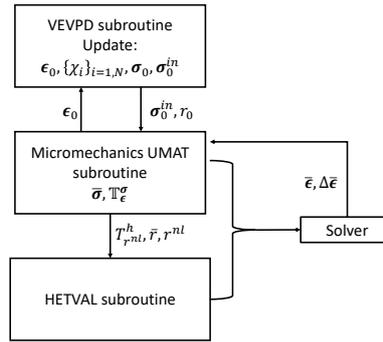
Figure 6: Flowchart of the numerical implementation in ABAQUS FE software for a composite structure. It should be mentioned that the HETVAL subroutine only needs  $T_n^{nl}$ , as the associated nonlocal tangent operator.
