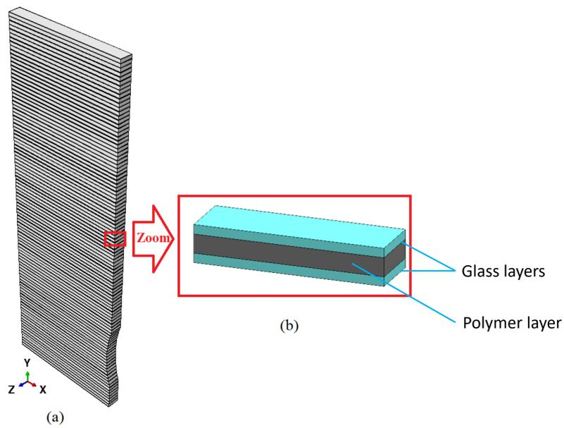
Figure 8: a) Multi-layered unilateral structure; b) zoom view and configuration of each RVE. The element type is the coupled temperature-displacement brick element (C3D8T).
