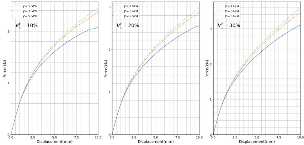
Figure 19: Force-displacement curves for the asymmetrically notched composite structure under  $5 \text{ mm s}^{-1}$  monotonic loading rate in different  $\gamma^{nl}$  with  $\xi^{nl} = 80 \text{ kN}$  when  $V_1^f = 10\%$ ,  $V_1^f = 20\%$ ,  $V_1^f = 30\%$ . The element type is the coupled temperature-displacement brick element (C3D8T).
