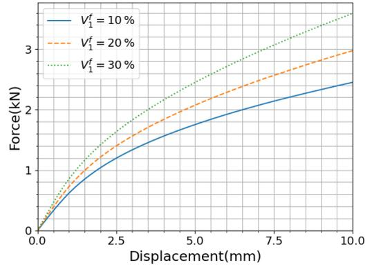
Figure 14: Force-displacement curves for the asymmetrically notched composite structure under  $5 \text{ mm s}^{-1}$  monotonic loading rate in different glass volume fractions ( $\gamma^{nl} = 5 \text{ GPa}$ ,  $\xi^{nl} = 80 \text{ kN}$ ). The element type is the coupled temperature-displacement brick element (C3D8T).
