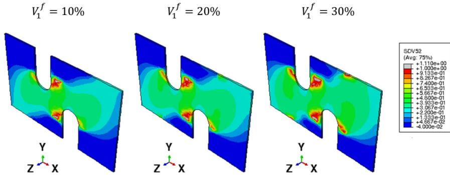
Figure 16: Damage profile under  $5 \text{ mm s}^{-1}$  monotonic loading rate using the nonlocal model for the asymmetrically notched structure with  $\gamma^{nl} = 5 \text{ GPa}$  and  $\xi^{nl} = 80 \text{ GPa}$  when  $V_1^f = 10\%$ ,  $V_1^f = 20\%$ ,  $V_1^f = 30\%$ . The element type is the coupled temperature-displacement brick element (C3D8T).
