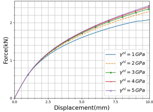
Figure 18: Force-displacement curves for the asymmetrically notched composite structure under  $5 \text{ mm s}^{-1}$  loading rate in different  $\gamma^{nl}$  with  $\xi^{nl} = 80 \text{ kN}$  when  $V_1^f = 10\%$ . The element type is the coupled temperature-displacement brick element (C3D8T).
