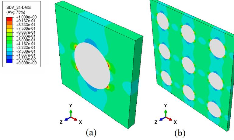
Figure 3: Damage profile under  $0.1 \text{ mms}^{-1}$  monotonic loading rate using the nonlocal model when  $l^{nl} = 0.1 l^\varepsilon$  in a) single short fiber reinforced RVE, b) a group of RVEs. Element size is set to  $0.05 \text{ mm}$ .
