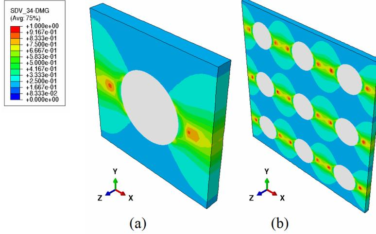
Figure 4: Damage profile under  $0.1 \text{ mms}^{-1}$  monotonic loading rate using the nonlocal model when  $l^{nl} = 100 l^e$  in a) single short fiber reinforced RVE, b) a group of RVEs. Element size is set to  $0.05 \text{ mm}$ .
