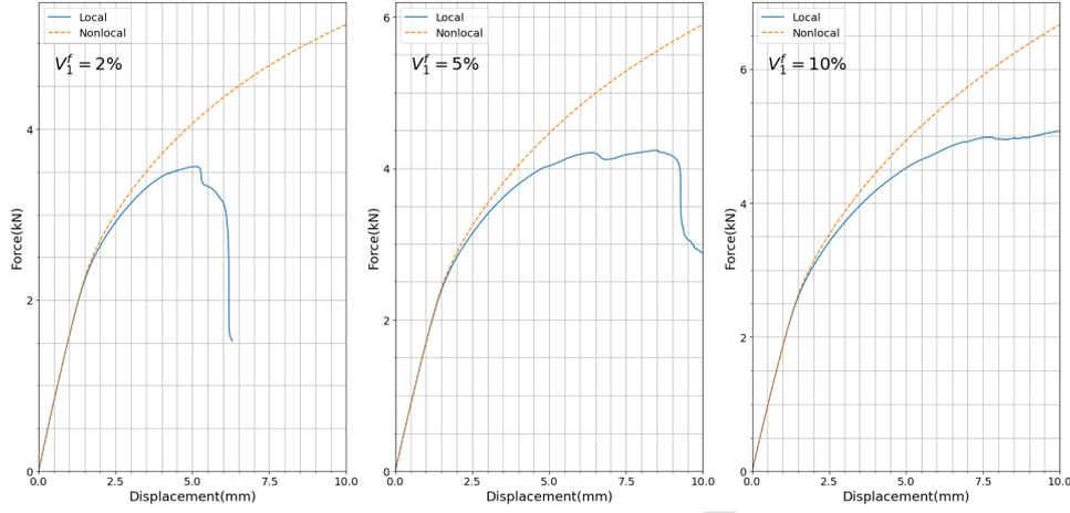
Figure 11: Force-displacement curves for the composite notched plate under  $5 \text{ mm s}^{-1}$  monotonic loading rate using local and nonlocal models with  $\xi^{nl} = 80 \text{ kN}$  and  $\gamma^{nl} = 5 \text{ GPa}$  when  $V_1^f = 2\%$ ,  $V_1^f = 5\%$ , and  $V_1^f = 10\%$ . The element type is the coupled temperature-displacement brick element (C3D8T).
