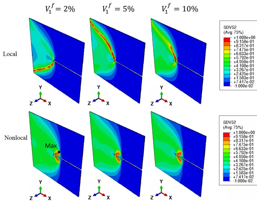
Figure 12: Matrix damage distribution in the notched plate under  $5 \text{ mm s}^{-1}$  monotonic tensile loading using local and nonlocal models with  $\xi^{nl} = 80 \text{ kN}$  and  $\gamma^{nl} = 5 \text{ GPa}$  when  $V_1^f = 2\%$ ,  $V_1^f = 5\%$ , and  $V_1^f = 10\%$ . The element type is the coupled temperature-displacement brick element (C3D8T).
