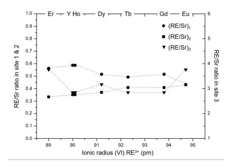
$\text{Ca}_{3}\text{RE}_{2}(\text{Si}_{3}\text{O}_{9})_{2}$  structure: repartition of Ca and RE in the 3 types of cationic sites
