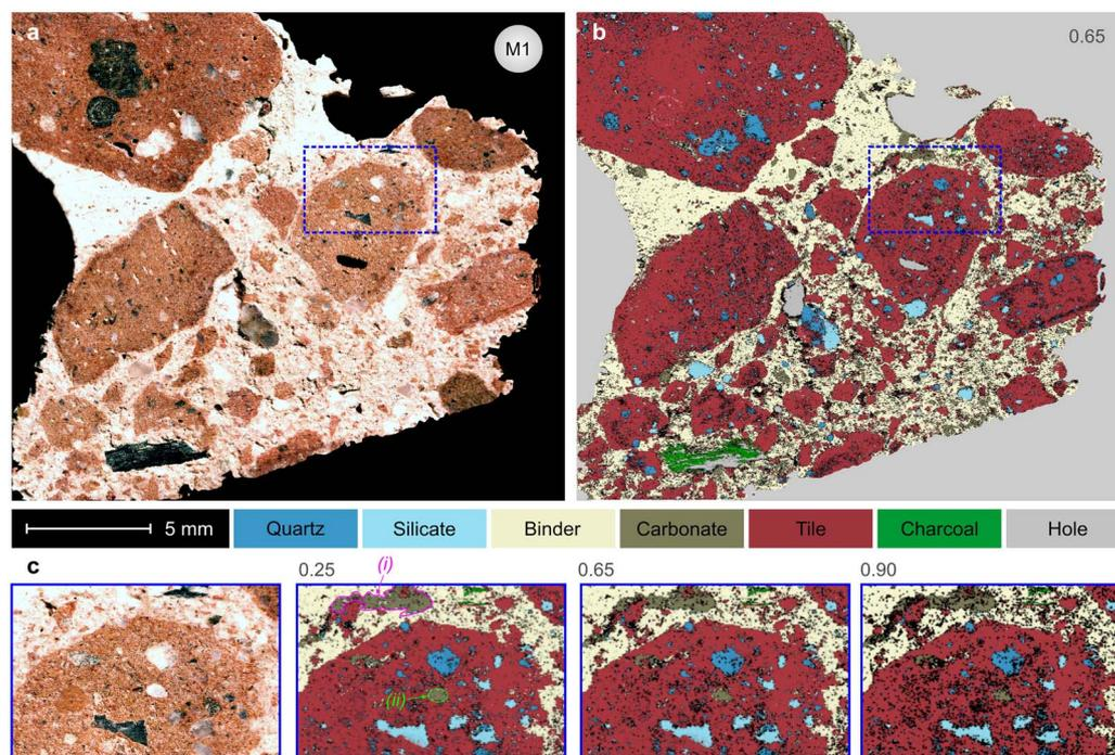
Fig. 7 Results provided by the ANN obtained on sample M1: (a) optical image of the sample surface. (b) ANN images of the seven detected categories (threshold value of 0.65). (c)  $\times 2.5$  zoom of the blue rectangle shown in (b) with various threshold values: 0.25, 0.65 and 0.90. The black pixels in (b) and (c) correspond to unidentified spectra.
