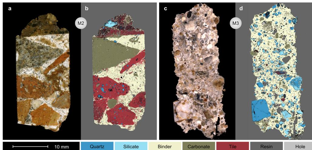
Fig. 8 Results provided by the ANN obtained on sample M2 and M3. Both samples were embedded in epoxy resin. (a) Optical image of the sample M2. (b) ANN images of M2 for the seven detected categories (threshold value of 0.65). (c) Optical image of M3. (d) ANN images of M3 for the detected categories (threshold value of 0.65). Note that the charcoal category is not displayed since it was not detected in both samples.
