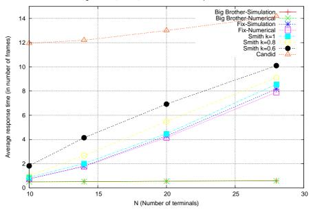
Load=0.8, gamma=15, beta=1, static method vs smith predictor vs candid method
