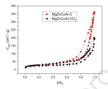
Fig.4. Adsorption/desorption isotherms of MgZnCoAl-CO<sub>3</sub> and MgZnCoAl-C.
