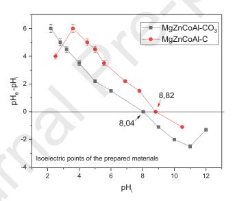
Fig.1. Isoelectric points of the prepared materials.
