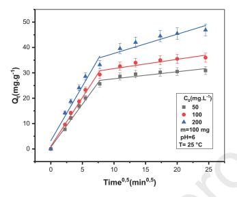
**Fig.10**. Data fitting of the nitrate adsorption kinetics by intra-particle diffusion model onto MgZnCoAl-C at different concentrations.
