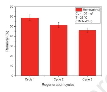
Fig.18: Regeneration study for MgZnCoAl-C at 1M NaOH
