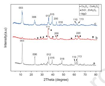
Fig.2. XRD patterns of (a) MgZnCoAl-CO<sub>3</sub>;(b) MgZnCoAl-C; (c) MgZnCoAl-NO<sub>3</sub>-
