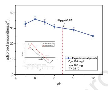
Fig 6. Effect of initial pH on adsorption of nitrate onto MgZnCoAl-C sample.
