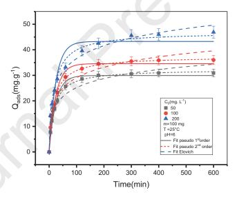
**Fig 9**. The curves representative of Nonlinear simulation of the pseudo-first-order (PFO), pseudo-second-order(PSO), and Elovich
