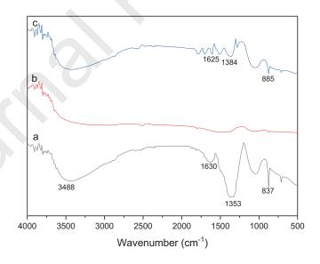
Fig.3. FTIR spectra for (a) MgZnCoAl-CO<sub>3</sub>, (b) MgZnCoAl-C, (c) MgZnCoAl-NO<sub>3</sub>
