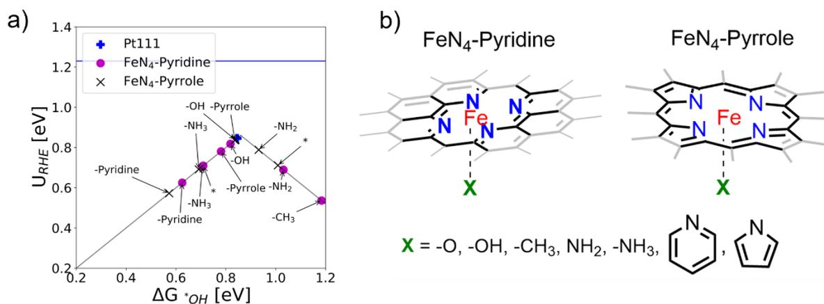
**Figure 7.** ORR activity volcano represented by O<sub>2</sub> reduction potential (RHE), U<sub>RHE</sub>, based on \*OH binding energies (ΔG\*<sub>OH</sub>) simulated on a series of FeN<sub>4</sub> pyridine and pyrrole sites with different axial ligands, and compared with Pt(111) (a). Schemes showing axial coordination in FeN<sub>4</sub>-Pyridine (left) and FeN<sub>4</sub>-Pyrrole (right), where X denotes the axial ligand (b). -\* denotes a pristine FeN<sub>4</sub> structure.
