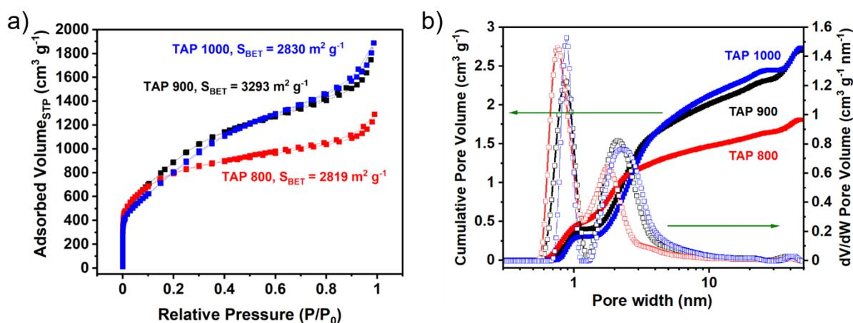
**Figure 2.** N<sub>2</sub> sorption isotherms with specific BET surface areas labelled (a) and corresponding pore size distributions and cumulative pore volumes calculated using 2D-NLDFT heterogeneous surface carbon model in SAIEUS software (b) of TAP-derived materials.
