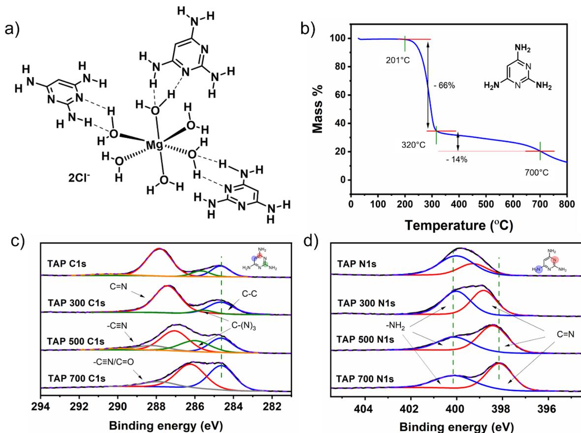
**Figure 1.** Representation of the self-assembly between 2,4,6-Triaminopyrimidine and MgCl<sub>2</sub>·6H<sub>2</sub>O (a). TGA curve of TAP (b). C1s (c) and N1s (d) XPS spectra of TAP pyrolyzed at 300, 500, and 700 °C.
