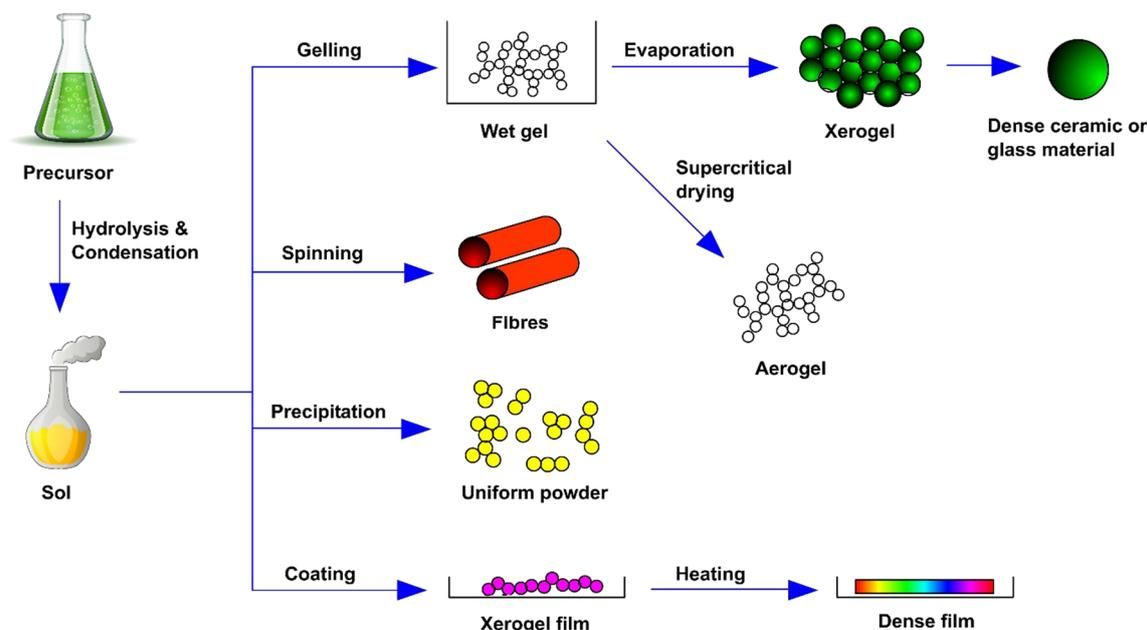
**Fig. 2** Methodologies of the sol-gel process for the synthesis of titanium dioxide materials. Gelling, spinning, precipitation and coating are the most common techniques used in the sol-gel process. Dense
