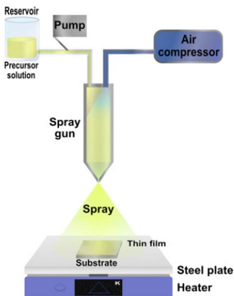
**Fig. 4** Spray pyrolysis. The spray gun provides the point for the substrate that was placed in the hot plate to get in contact with the precursor solution. Licensed from Elsevier books “Nanosensors for smart cities”, Han et al. (2020)
