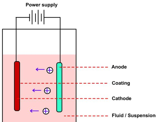
**Fig. 3** Cathodic electrophoretic deposition cell (Srikanth et al. 2017). The photocatalyst is suspended in the solvent phase with a steady direct voltage (25–400 V). Electrolysis produces ions, which migrate towards the oppositely charged electrode as a result of electrophoresis and gets deposited over the electrode support
