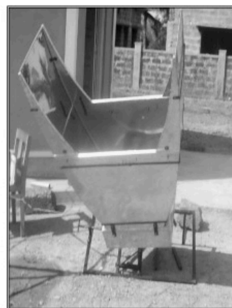
Photograph of box cooker implemented with CPC-30 collector
