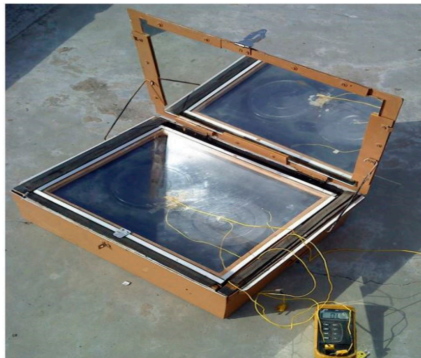
Figure 10. Schematic diagram of solar cooker SFSC. Reprinted/adapted with permission from Ref. [38], 2012, Elsevier.
