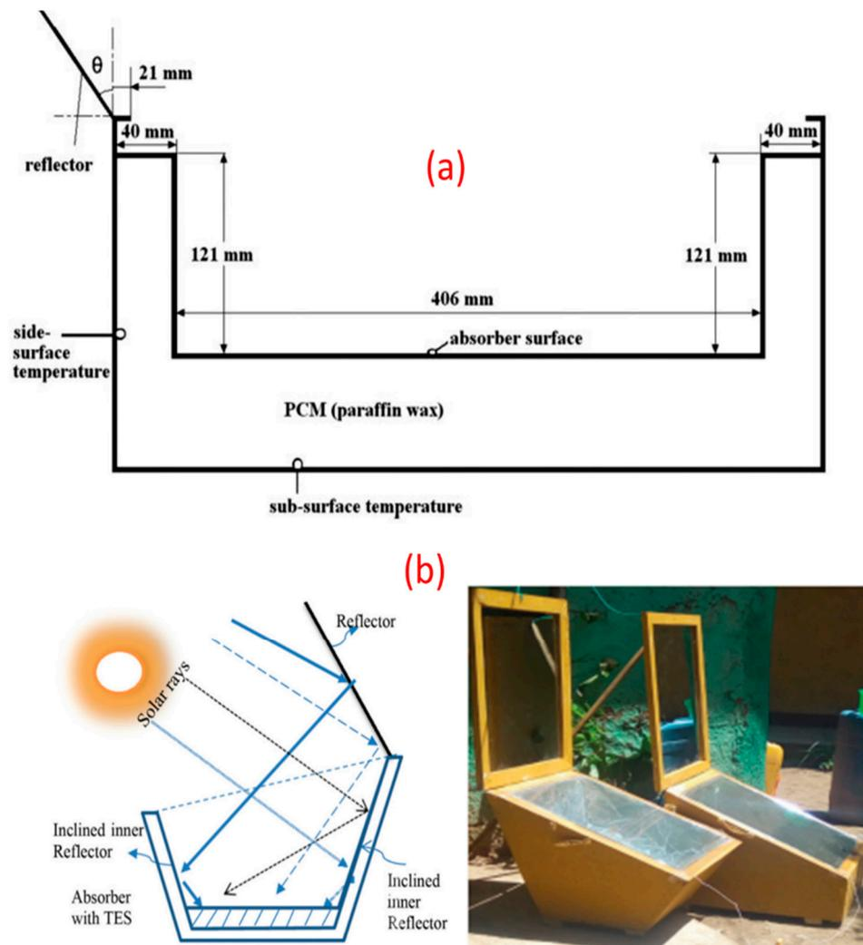
**Figure 23.** (a) Schematic diagram; (b) Experiment setup of box-type SC. Reprinted/adapted with permission from Ref. [55], 2012, AIP Publishing and Ref. [67], 2021, Taylor & Francis online Publishing.
