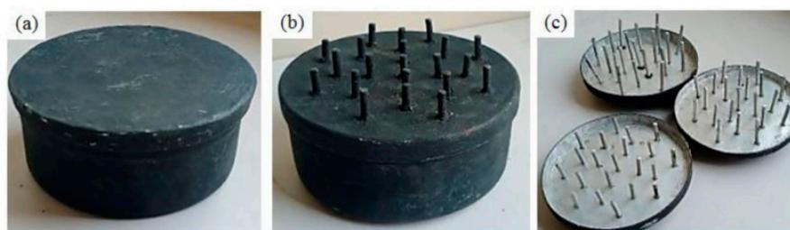
**Figure 16.** Diagram of fins of varying sizes used over vessels. (a) Without fins; (b) Finned cooking vessel; (c) Finned lids (inside view). Reprinted/adapted with permission from Ref. [45], 2021, Elsevier.
