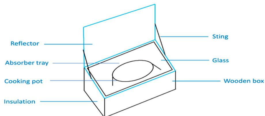
**Figure 2.** Schematic of box-type solar cooker.
