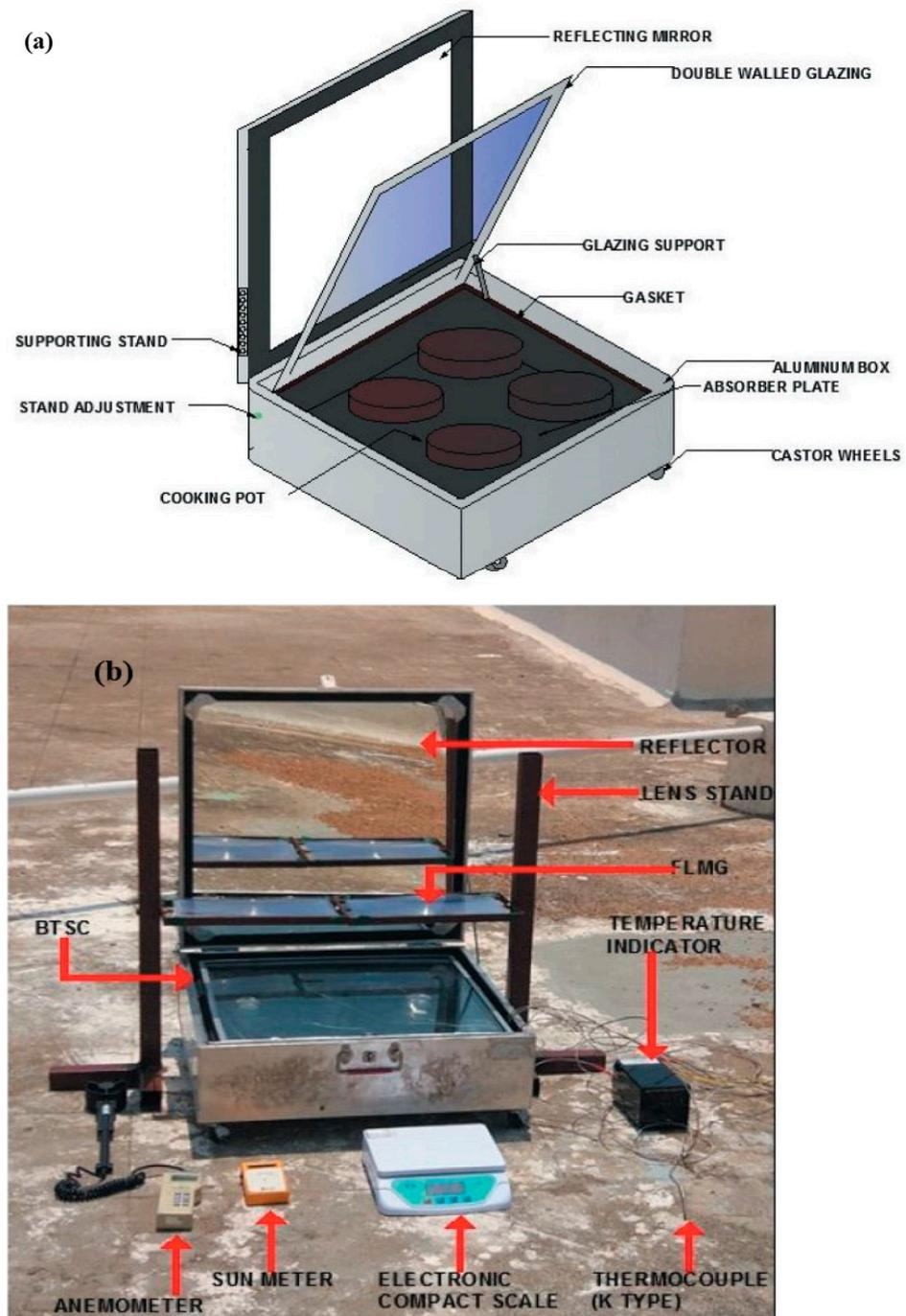
**Figure 13.** (a) Components of box-type solar cooker; (b) Experimental setup Mirror. Reprinted/adapted with permission from Ref. [41], 2020, Taylor & Francis online.
