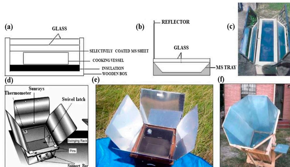
**Figure 6.** Pictures of solar cooker developed: (a) Simple box with glazed glass lid and insulated bottom; (b) Single-reflector box-type solar cooker; (c) Twin-reflector solar cooker; (d) Simple four-faced-reflector solar cooker; (e) Four-faced-reflector solar cooker with Swinging rack; (f) Multi-faced conical reflector solar cooker. Reprinted/adapted with permission from [8], 2010, Elsevier.
