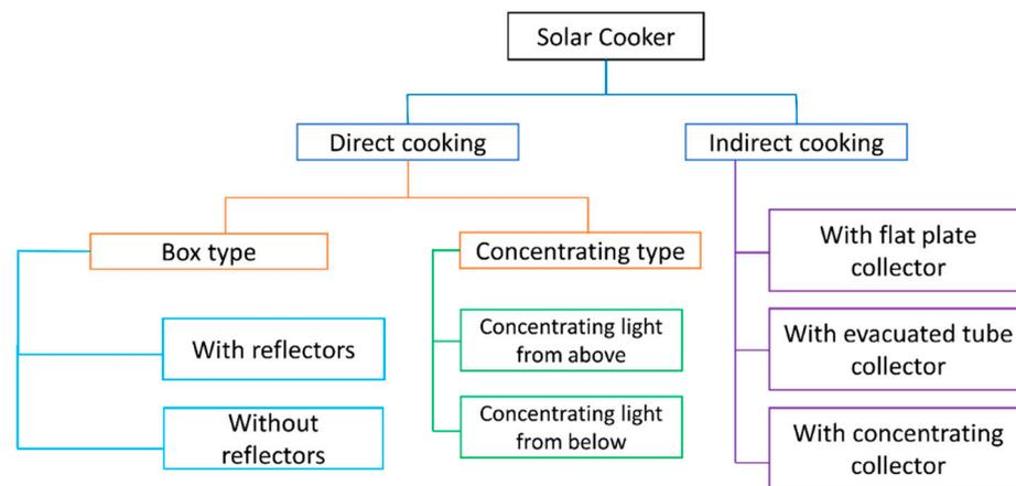
**Figure 1.** Classification of solar cooker. The temperature attained in the box type is medium (approx. 120 °C) [17] and very high in concentrating type (approx. 290 °C); however, indirect cooker has a high temperature but with a control option. Reprinted/adapted with permission from Ref. [18], 2018, Elsevier.
