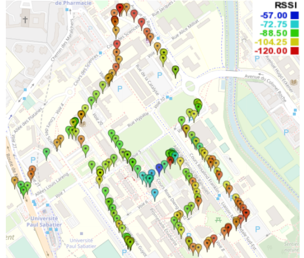
Figure 5: GPS Coordinates Transmitted With RN2483 Equipped With Xbee GPS Module
