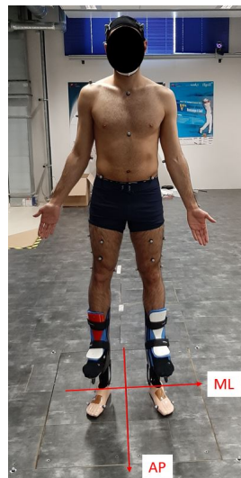
Figure 2. Subject wearing the prosthetic simulators with prosthetic feet + feet frame.
