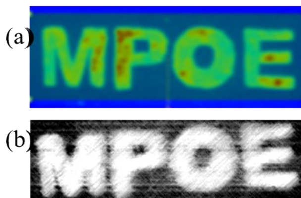
Figure 8. (a) Persistent luminescence image from the “MPOE” pattern, hand painted using \text{ZGSO}:\text{Ni}^{2+} , \text{Er}^{3+} , \text{Cr}^{3+} NPs detected with Si-based visible camera; (b) persistent luminescence image from the “MPOE” pattern, hand painted using \text{ZGSO}:\text{Ni}^{2+} , \text{Er}^{3+} , \text{Cr}^{3+} NPs, detected with InGaAs-based NIR camera.
