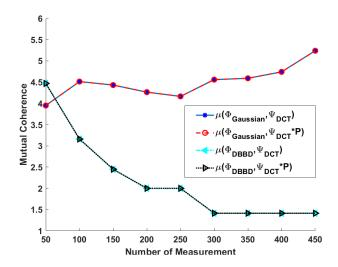
FIGURE 4. Impact of proposed encryption on mutual coherence.
