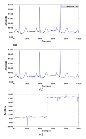
FIGURE 3. Recovery via adaptive dictionary learning (MOD) with and without actual key. (a) Initial ECG signal (plaintext). (b) Recovery of ECG Signal on user-side with the true key PRD = 0.09%, SNR = 60.4dB. (c) Recovery of the ECG signal in cloud-side with the wrong key PRD = 150%. SNR = -3dB.
