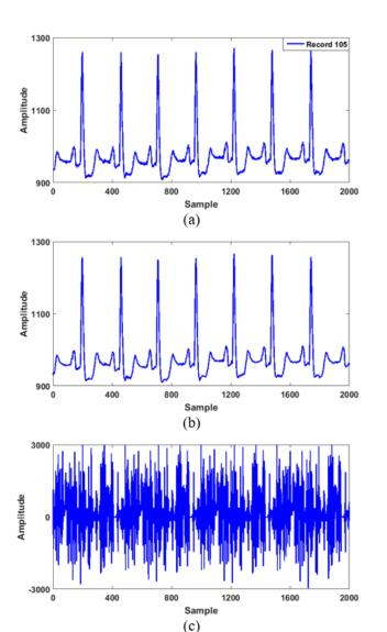
FIGURE 2. Recovery of ECG signal via DCT dictionary with and without actual key. (a) Initial ECG signal (plaintext).(b) Recovery of ECG Signal on client-side with the actual key (PRD = 0.29%, SNR = 50.6dB). (c) Recovery of the ECG signal in cloud-side with the wrong key  $(PRD = 10^6\%, SNR = -30.22dB)$ .
