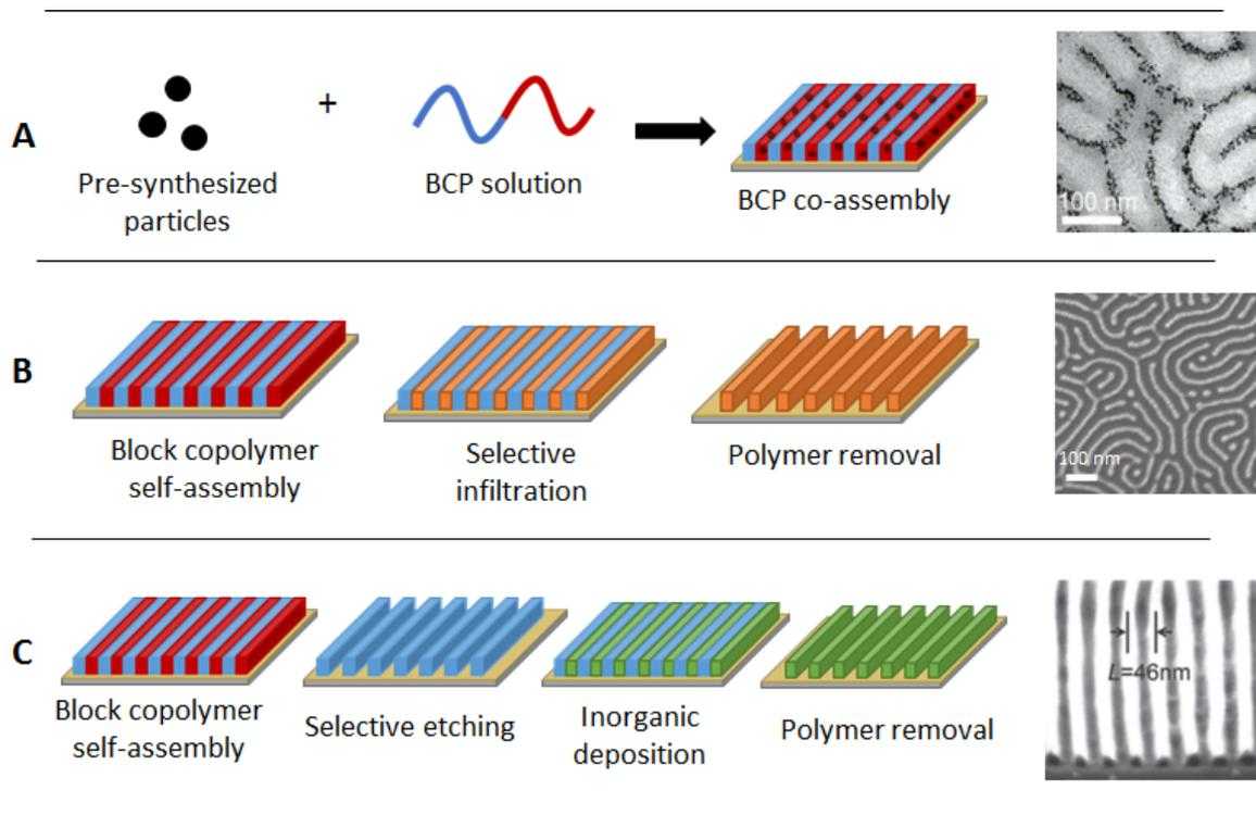
**Figure 7.** Schematics of the different strategies followed to design optical metamaterials architectures using BCP films as a template: A) BCP co-assembly (Reproduced with permission<sup>[169]</sup>; Copyright 2008 Wiley-VCH) B) selective infiltration, (Reproduced with permission<sup>[68]</sup>, Copyright 2019 Royal Society of Chemistry) and C) Inorganic deposition, (Reproduced with permission<sup>[169]</sup>, Copyright 2014 Wiley-VCH).
