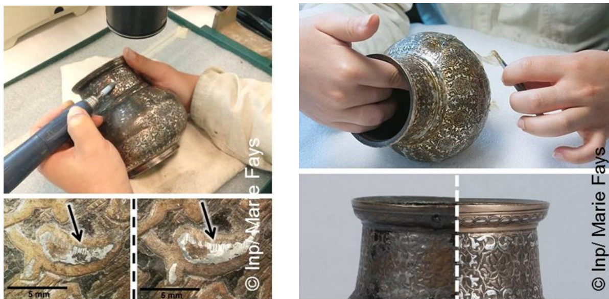
Figure 5.a. Nettoyage aux polissoirs, b. Nettoyage aux gels.
