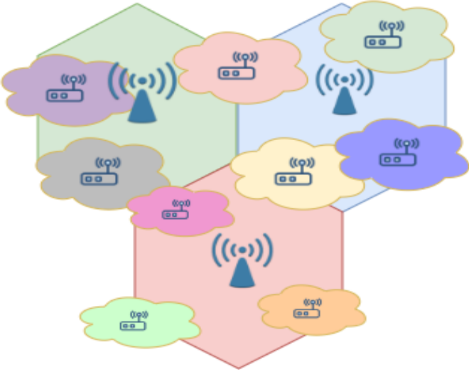
Fig. 1. A vertically integrated cellular WiFi system with M = 3 macro cells and W = 9 overlapping WiFi access points.
