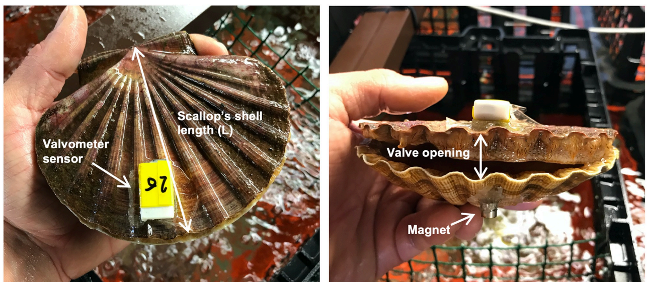
Fig 1. Positioning of Hall effect sensors and magnets on scallops. Schematic view of a scallop equipped with a valvometer sensor.
