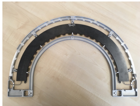
Figure 13.13: A prototype half-ring in its aluminium handling and transport frame.
