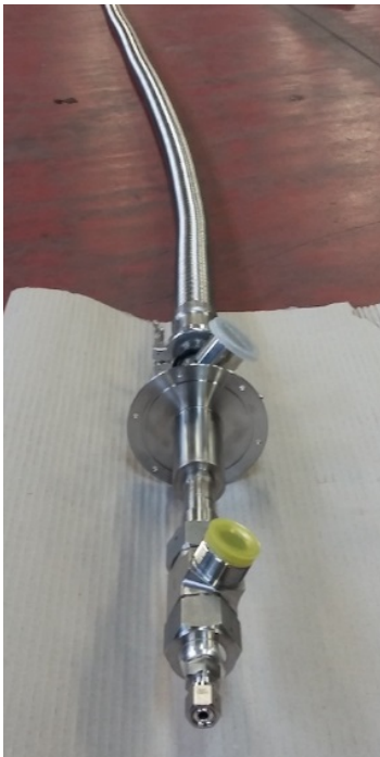
Figure 15.7: Left: Picture of the 5 kW ITk flex line. Right: Longitudinal cross-section of the 50 mm ITk flex line.
