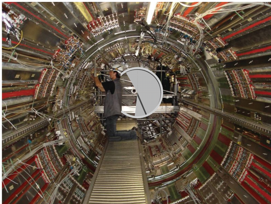
Figure 18.9: The bore of the Solenoid vacuum vessel during installation, with a sketch of a possible shielding disk (consisting of two half disks) superimposed. The disks can be rotated to either allow work in a segment up to 180^\circ , or to cover the whole area for maximum protection.
