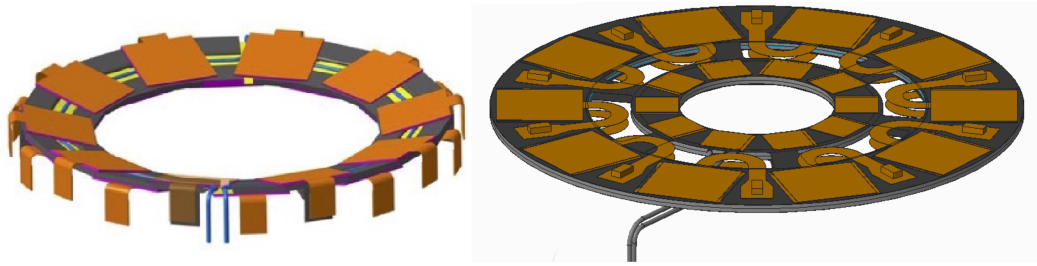
Figure 13.7: Ring layouts in the “Inclined Inner” (left) and “Inner Alternative” (right) proposals. Modules are depicted as orange rectangles.
