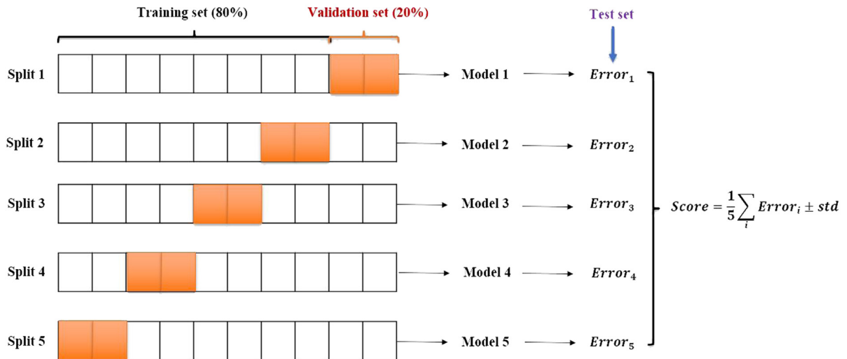
Fig. 13. Flow chart of the 5-fold cross validation used in this paper.
