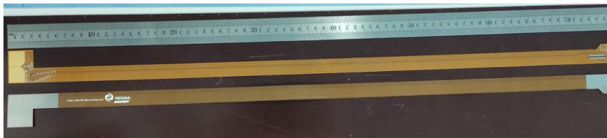
Figure 7.10: A 4-layer flex cable prototype from Shennan Circuits company in China
