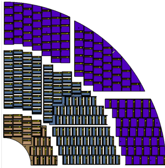
Figure 7.16: Detector units with modules assembled on the inner, middle and outer support plates
