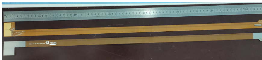
Figure 7.10: A 4-layer flex cable prototype from Shennan Circuits company in China
