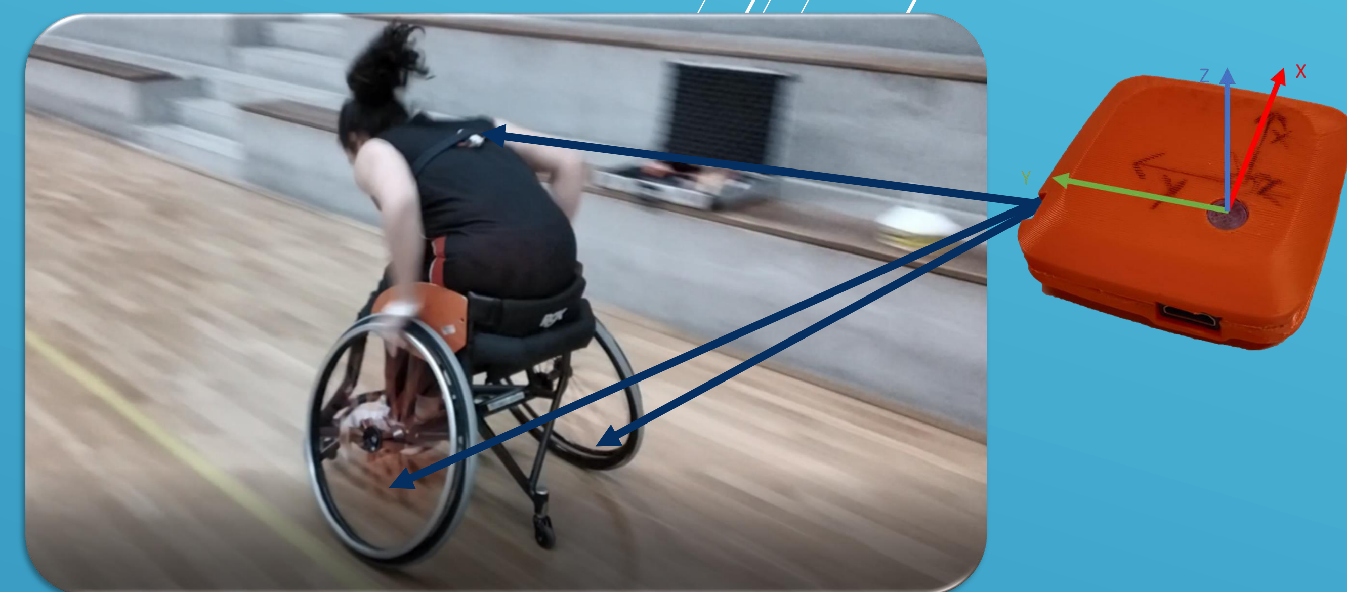
Figure 1 : Female wheelchair basketball player during a sprint with 3 IMUs.
