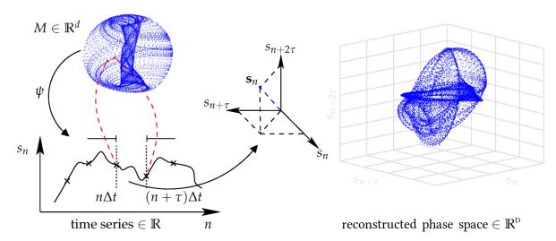
Figure 3: Illustration of the concept of the Delay-Embedding theorem. Reproduced with permission from Ana González-Marcos [21]
