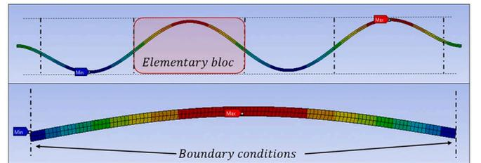
Fig. 2. Elementary block for studying flexural modes.
