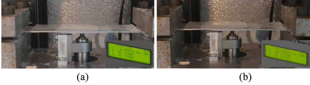
Fig. 20. Side view of the regular sample for a 0.45 mm long displacement (a) and a 1 mm long displacement (b).
