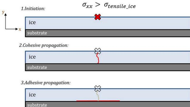
Fig. 4. Fracture mechanism for low-frequency flexural modes.
