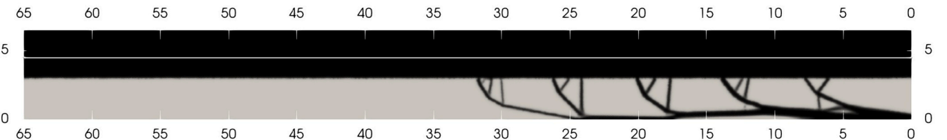
Fig. 24. Optimized design computed for the clamped configuration. The blank line indicates the substrate-ice interface.
