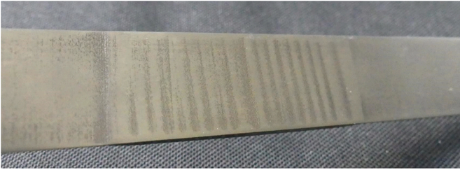
Fig. 29. Non plan surface of the substrate highlighted after polishing.
