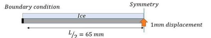
Fig. 3. Reduced static beam model used for computations.
