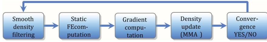
Fig. 22. Flowchart of the topology optimization algorithm.
