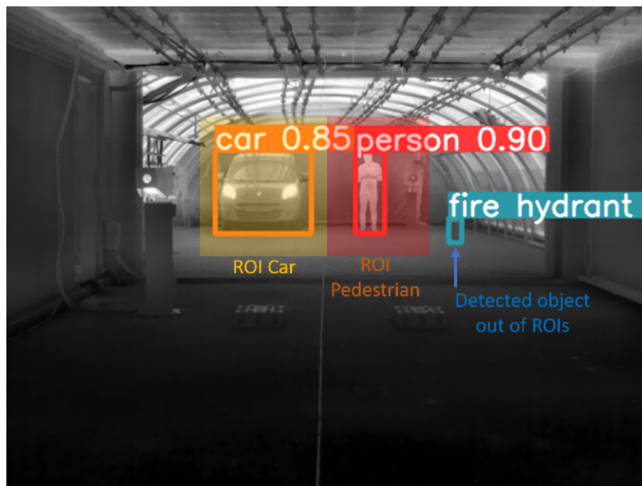
Figure 23. Example of output obtained from YOLOv5 and application of ROIs for discrimination in object detection.
