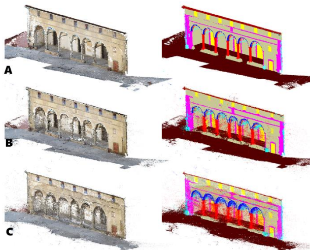
Figure 9: Back-Projection results for 2_OSA : A) ground-truth point cloud, B) image ground-truth reconstruction, C) prediction reconstruction.
