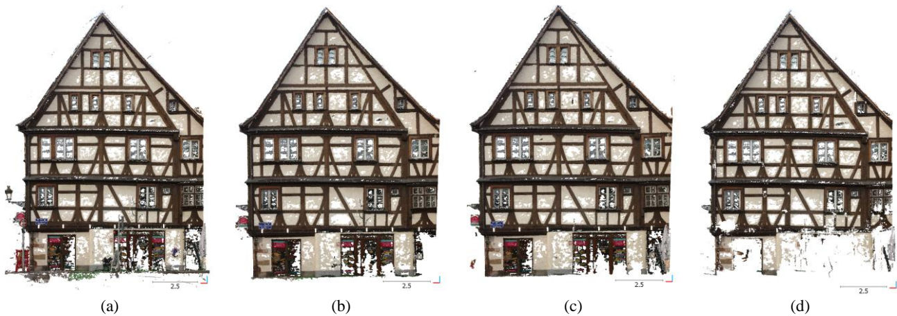
Figure 5. Dense point cloud results from (a) raw dense matching without noise cleanup, (b) manual cleaning on CloudCompare, (c) automatic noise exclusion via manual image masks and (d) automatic noise exclusion via AI-created image masks.
