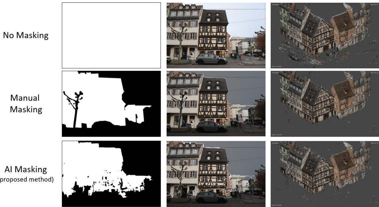
Figure 2. Illustration of the proposed workflow and comparison with traditional manual masking of unwanted objects. The third column shows the resulting dense point clouds.
