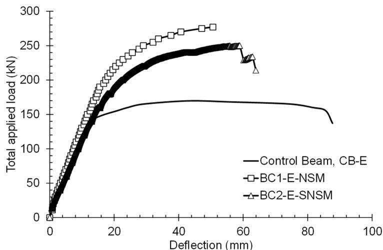
Fig.4: Load deflection curve of tested beams
