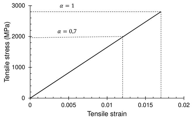
Fig.13: Constitutive model of CFRP reinforcement
