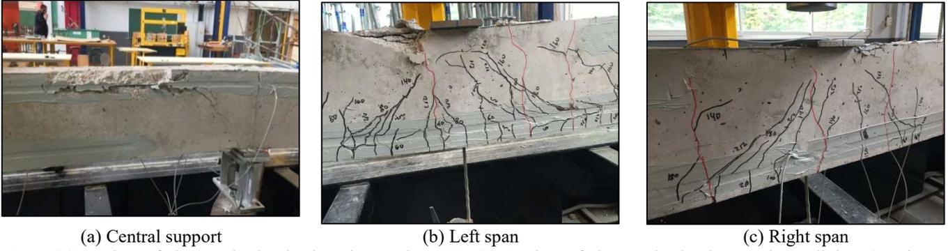
Note: (1)Number of the cracks in the hogging region: 28; (2)Number of the cracks in the sagging region (maximum number): 47
