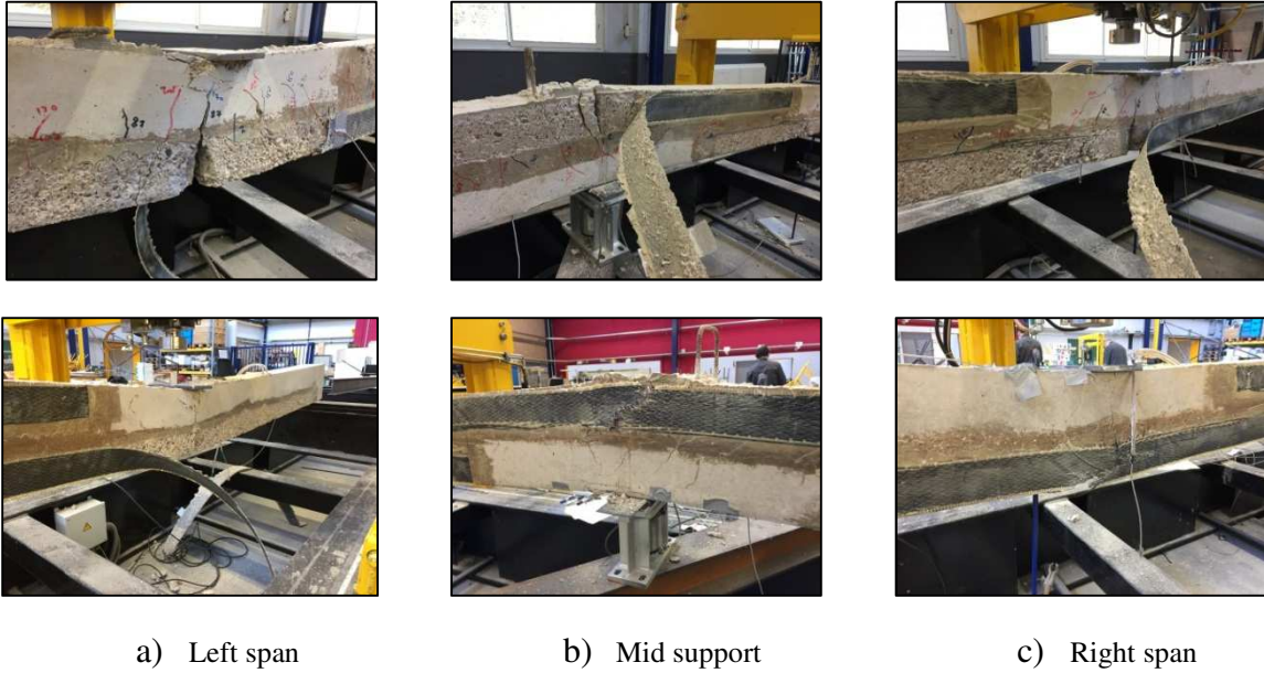
Fig. 14: Failure mode of beam BC5-EB1S-weight(700)
