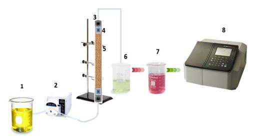
**Figure 1.** Schema of the experimental setup for the Cr(VI) fixed-bed adsorption. 1—Cr(VI) solution reservoir, 2—Peristaltic pump, 3—Cotton plugs, 4—Glass ball, 5—RPS fixed bed, 6—taken sample of Cr(VI), 7—Ready sample for analysis, 8—Spectrophotometer UV-Visible.
