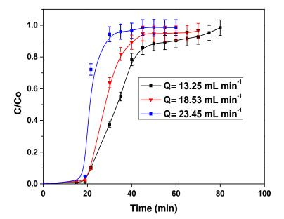
Figure 7. Effect of the flow rate on breakthrough curves.
