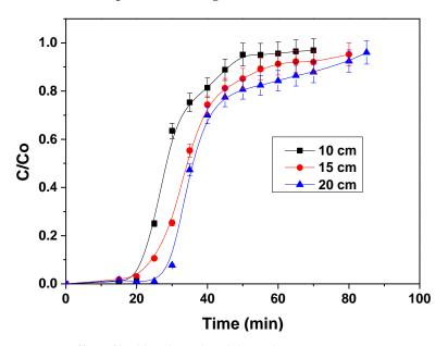
Figure 6. Effect of bed height on breakthrough curves.
