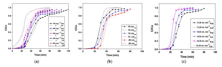
**Figure 8.** A comparison of the experimental and predicted breakthrough curves obtained at different initial Cr(VI) concentrations (**a**), different bed heights (**b**) and different flow rates (**c**), according to the Bohart-Adams model.
