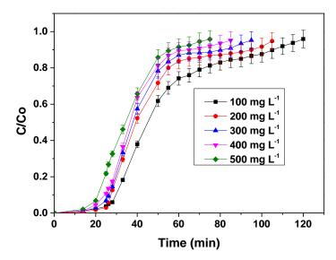
Figure 5. Effect of initial concentration on breakthrough curves.
