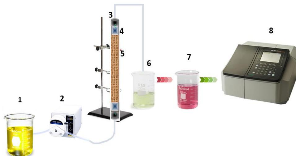
**Figure 1.** Schema of the experimental setup for the Cr(VI) fixed-bed adsorption. 1—Cr(VI) solution reservoir, 2—Peristaltic pump, 3—Cotton plugs, 4—Glass ball, 5—RPS fixed bed, 6—taken sample of Cr(VI), 7—Ready sample for analysis, 8—Spectrophotometer UV-Visible.
