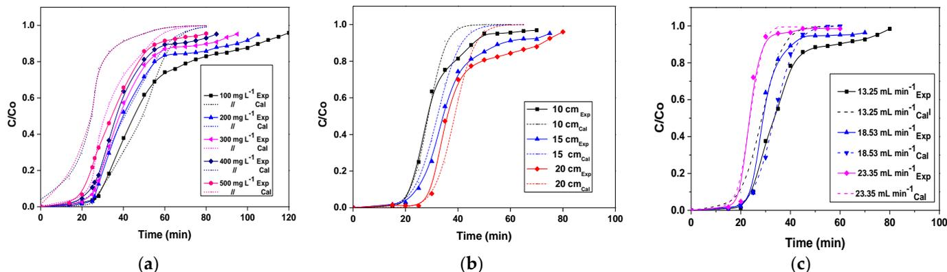
**Figure 8.** A comparison of the experimental and predicted breakthrough curves obtained at different initial Cr(VI) concentrations (a), different bed heights (b) and different flow rates (c), according to the Bohart-Adams model.
