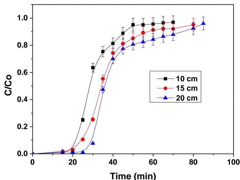
Figure 6. Effect of bed height on breakthrough curves.
