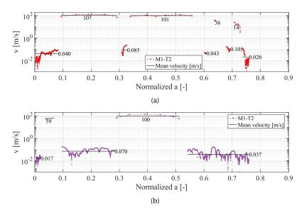
Fig. 8: Crack tip speed (v)  $[m.s^{-1}]$  as a function of the normalized crack length (a) [mm]. Black bars present the phase-dependent mean velocity  $[m.s^{-1}]$ .
