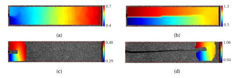
Fig. 6: Identified displacement field [mm] and corresponding Williams' series projection [mm] within the domain surrounding the crack-tip (defined by  $R_{min}$  and  $R_{max}$ ) of the first and last recorded image for experiment M2-T15. The used Williams' series parameters are listed in Table 3.
