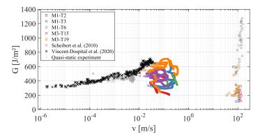
Fig. 15: Energy release rate (G)  $[J.m^{-2}]$  as a function of velocity (v)  $[m.s^{-1}]$  for the alternate cracking and one entirely quasi-static experiment.
