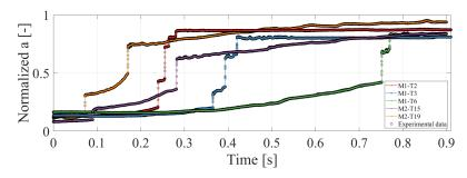
Fig. 7: Normalized crack length (1.0 = 63 mm) as a function of recording time [s] for all five experiments.
