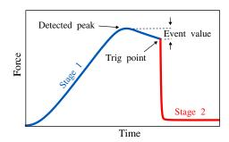
Fig. 4: Example of stage change method (Static Crack Detection).
