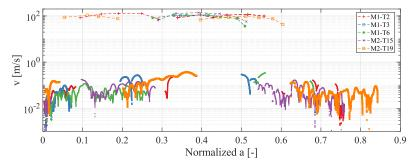
Fig. 11: Velocity  $[m.s^{-1}]$  as a function of the normalized crack length [mm] for all conducted experiments.
