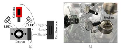
Fig. 5: Experimental setup: (a) sketch, (b) picture.
