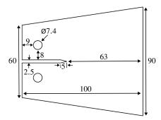
Fig. 3: Sample geometry [mm].
