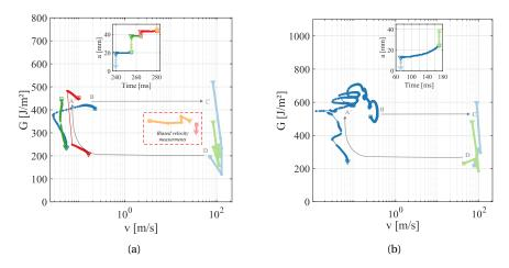
Fig. 14: Energy release rate (G)  $[J.m^{-2}]$  as a function of velocity (v)  $[m.s^{-1}]$  for the alternate cracking phases with its corresponding temporal evolution of the crack for: (a) M1-T2 and (b) M2-T19. Reference to the phases of the theoretical kinematic law (see Figure 1) are added for better comprehension.
