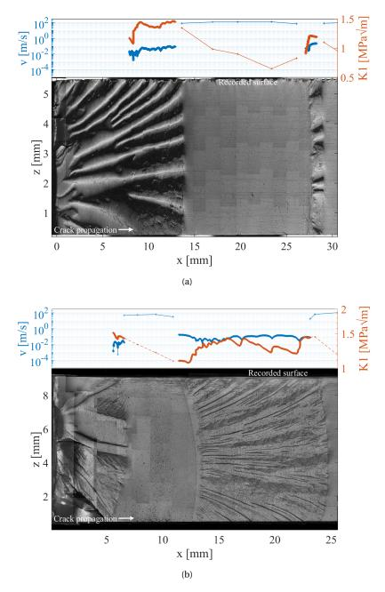
Fig. 12: Velocity [m.s<sup>-1</sup>] and K<sub>I</sub> [MPa $\sqrt{m}$ ] as a function of crack length [mm] in face with the microscopic image of the fracture surface for the experiments: (a) M1-T2 and (b) M2-T15. A spatial matching error between DIC and microscope measurements of ~160  $\mu$ m and ~140  $\mu$ m has to be considered for M1-T2 and M2-T15, respectively.
