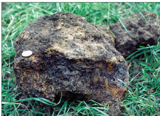
Fig 2. A slag block from Moore's Farm (note charcoal).
