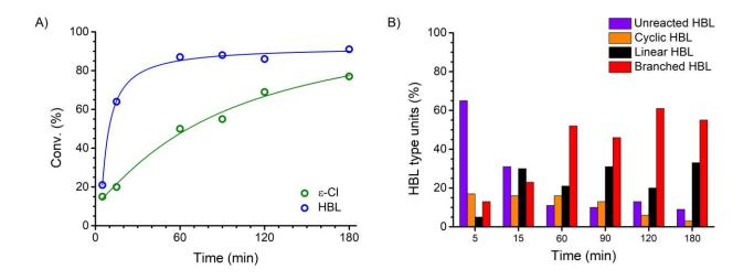
Figure 2: kinetic study A) conversion of ε-CL and HBL vs time B) Type of HBL motive vs time.
