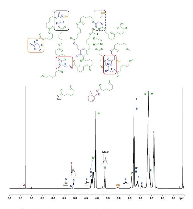
Figure 1: <sup>1</sup>H NMR spectrum and proposed structure of HBL/ε-CL copolymers (Table 1, run 4).
